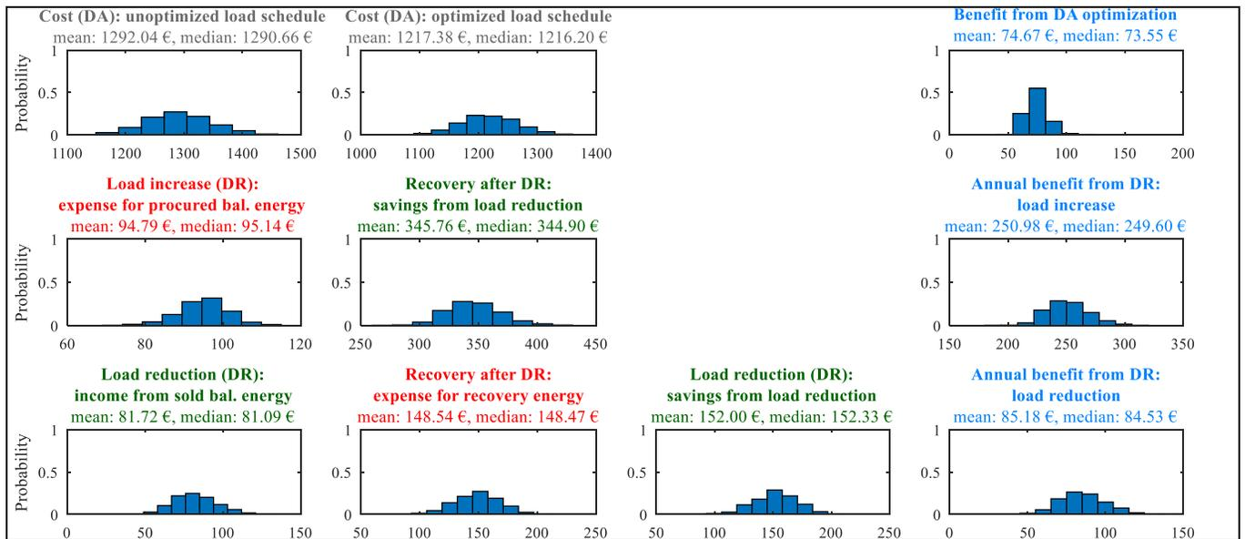
Figure 4. Probability histograms of the modeled cash flow positions (red – positive, green – negative, blue – total) with day-ahead rescheduling.
