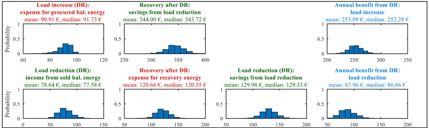
Figure 3. Probability histograms of the modeled cash flow positions (red – positive, green – negative, blue – total) without day-ahead rescheduling.
