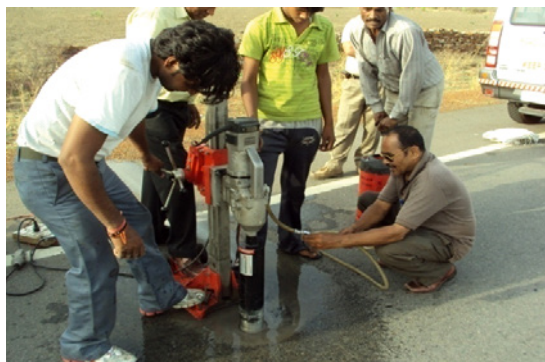
Figure 6. Full-depth core cutting of bituminous layers
