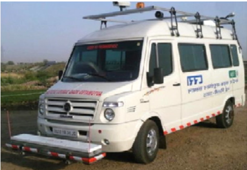
Figure 3. Network survey vehicle with different components
