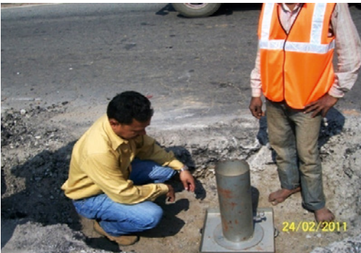
Figure 5. Field density test
