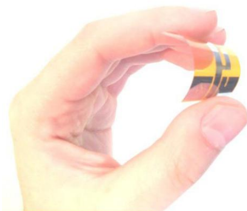
A Flexible Antenna for Integration within Wearable Wireless Systems. (Photo by Haider Raad ©)
