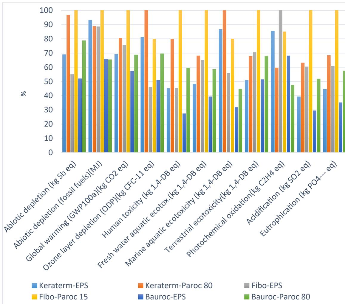
**Figure 1.** Impact of masonry walls (1m<sup>2</sup>) according to the method: CML-IA baseline V3.04.
