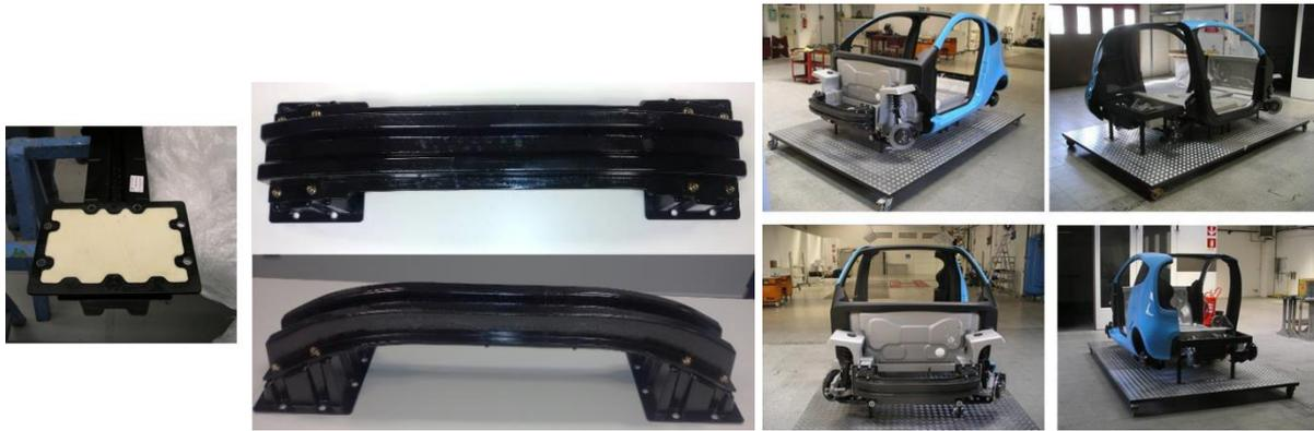
Figure 3.29. Evolution Front Bumper Crossmember demonstrator prototype and the technological mock-up with integrated demonstrators
