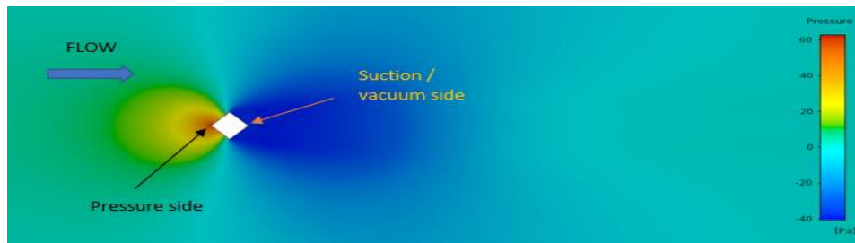
Fig. 3.2. Concept of zones for a diamond ( 45 \times 45 ) prism at constant speed of 10 m/s.
