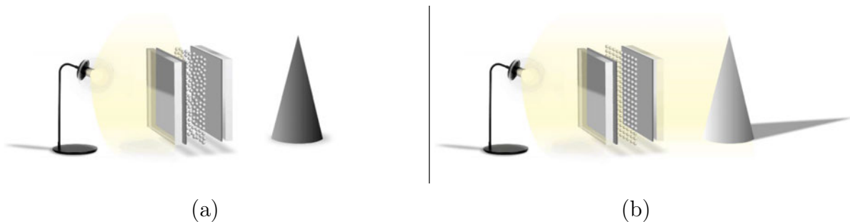
Fig. 2.3. (a) - When off, particles are scattered creating opacity for privacy, shading, solar control, or video projection, (b) - when on, particles align, creating transparency for an open atmosphere and natural light [89].
