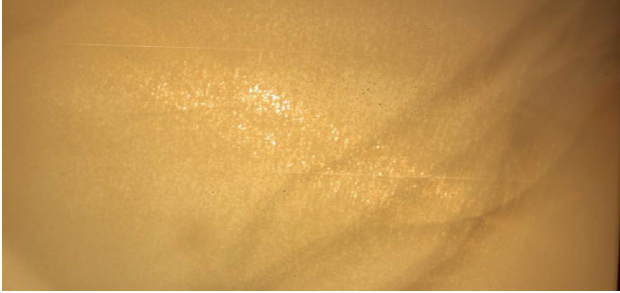
Fig. 5.8. Unswitchable (stuck) LC cluster before temperature treatment. Darker, brighter and transparent spots resemble inhomogeneities of polyimide coating.
