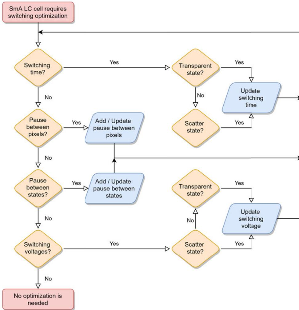
Fig. 2.20. *SmA LC* cell switching optimization diagram.
