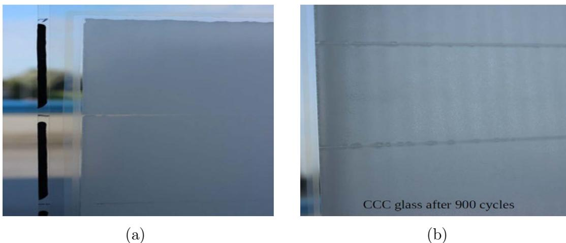
Fig. 2.16. *SmA LC* cell ( $8 \times 1$  design): (a) — close-up of pixels laser ablation lines and outline; (b) — close-up of pixels, active areas and laser ablation lines.
