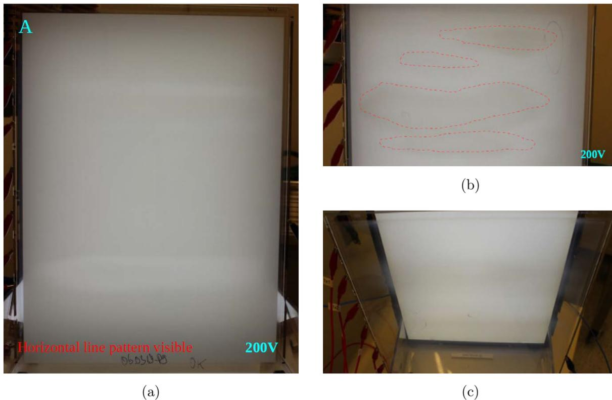
Fig. 2.17. *SmA LC* cell ( $8 \times 1$  design): (a) — close-up of the scatter state; (b), (c) — close-up of the transparent state. Additional background (behind the *LC* cell) lightning was used for better visual defect identification.
