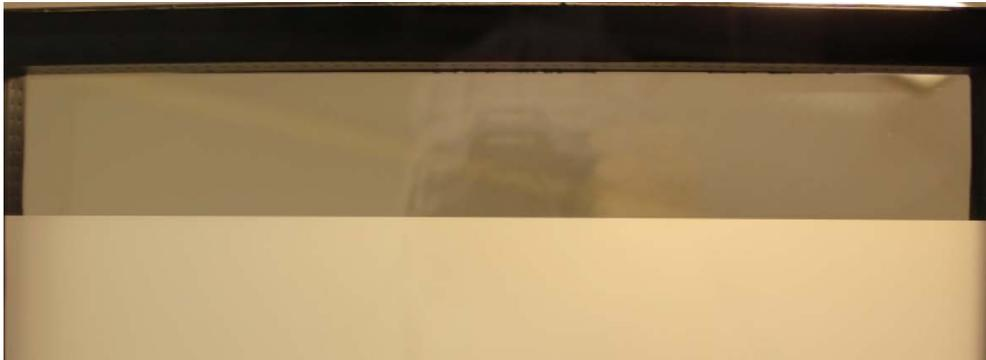
Fig. 2.19. Unswitchable (stuck) *LC* cluster zones disappeared after testing cycle and parameter optimization.
