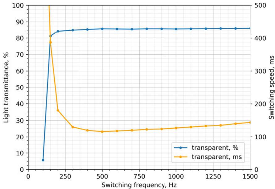
Fig. 2.10. Switching speed (orange) and light transmittance (blue) at different switching frequencies during transition to transparent state.
