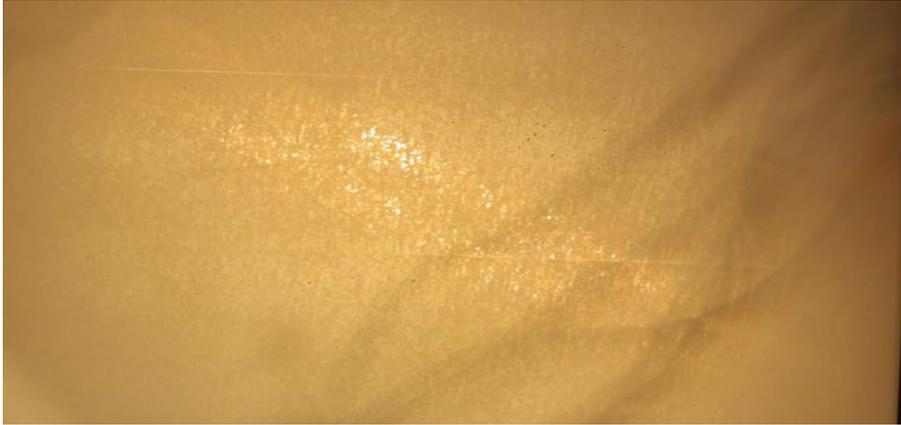
Fig. 2.25. Unswitchable (stuck) *LC* cluster before temperature treatment. Darker, brighter and transparent spots resemble inhomogeneities of polyimide coating.
