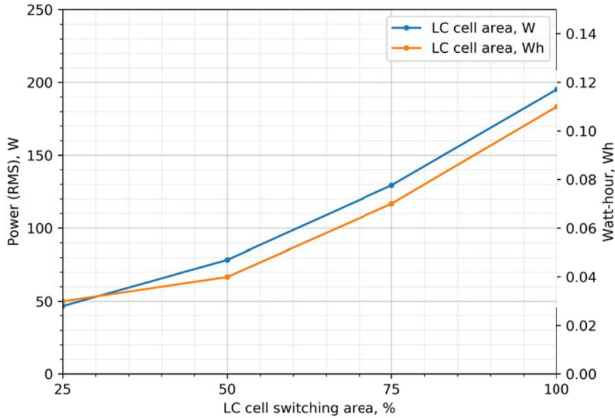
Fig. 2.12. Consumed power (*RMS*) based on the *LC* cell's switching area.
