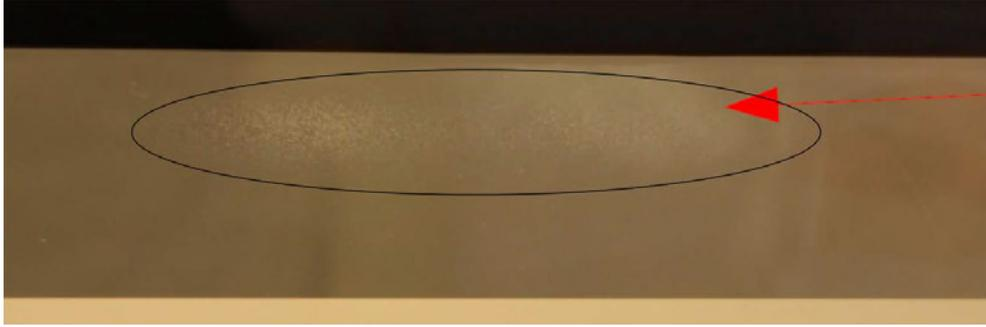
Fig. 2.18. Unswitchable (stuck) *LC* cluster zones in inner state before testing cycle and parameter optimization.
