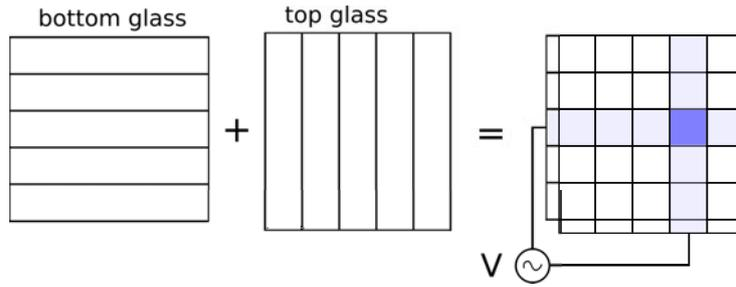
Fig. 2.4. Simplified schematic representation of passive matrix driving technique.
