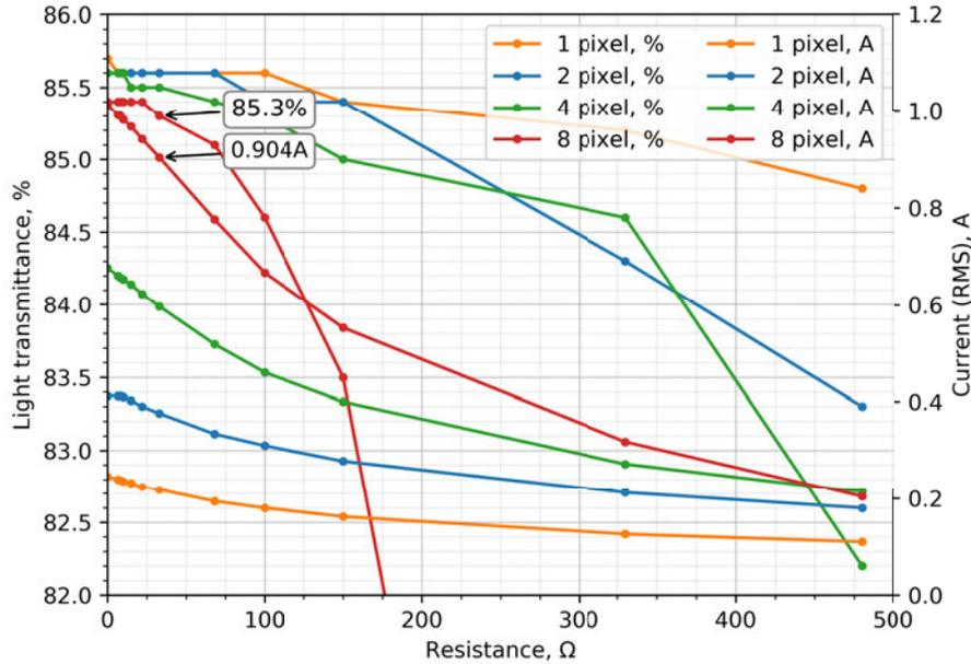
Fig. 2.13. Current measurements with current limiting resistors.
