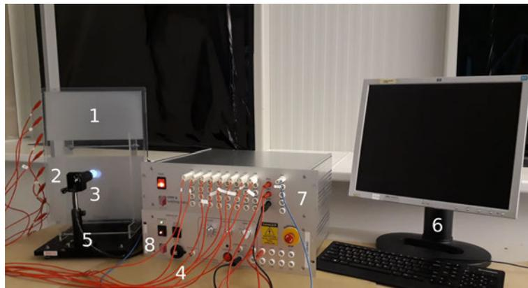
Fig. 2.7. Overview of the experimental setup used for functional testing of *SmA LC* cells.
