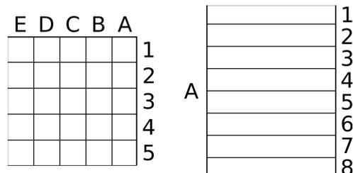
Fig. 2.3. Graphical representation of *LC* cell physical design types. On the left -  $5 \times 5$  pixel and on the right  $8 \times 1$  design.
