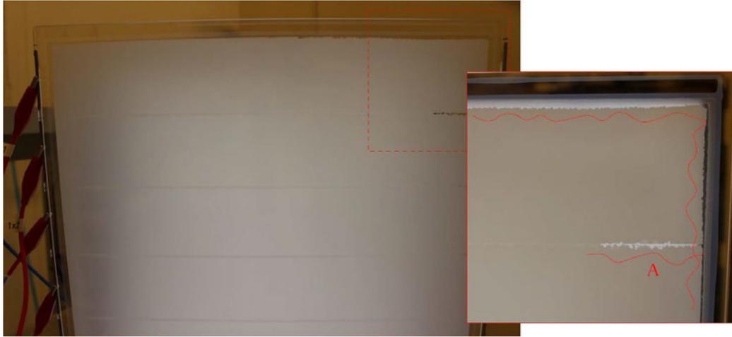
Fig. 2.21. Defected *SmA LC* cell — pixels with wavy outline, rugged edges and unfixable separation line between two pixels.
