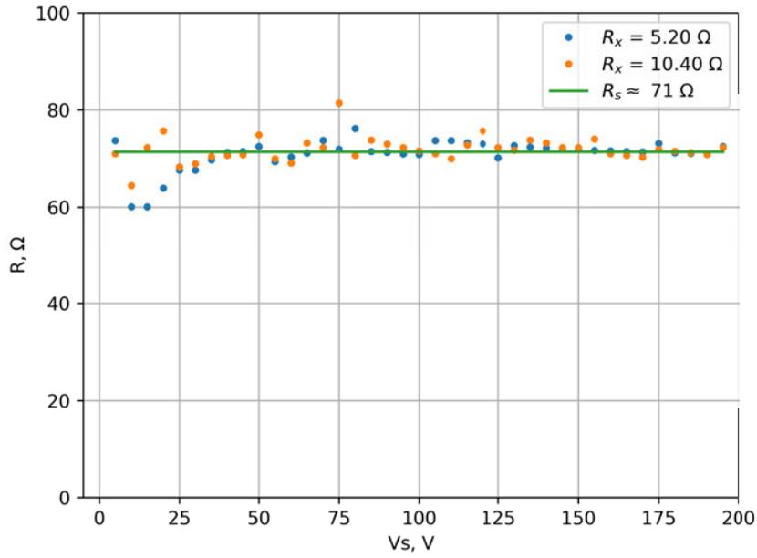
Fig. 2.28. Equivalent series resistance  $R_S$  dependence of  $V_S$ .
