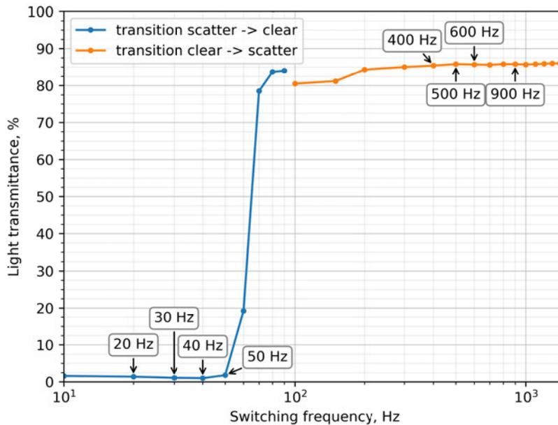
Fig. 2.8. Light transmittance at different switching frequencies.
