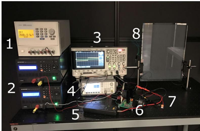
Fig. 2.23. Overview of the experimental setup used for switching waveform optimization for *SmA LC* cells. Used equipment: 1 – Agilent U8032A; 2 – B&K Precision 9184; 3 – Agilent DSOX2014A; 4 – Agilent 33500B; 5 – Tektronix P5200; 6 – Apex PA93; 7 - textitRx (current measurement resistor), 8 – *SmA LC* cell.
