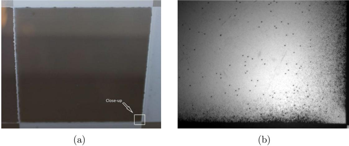
Fig. 2.15. *SmA LC* cell ( $5 \times 5$  design): (a) — close-up of the middle pixel *C3*; (b) — close-up of the lower right corner of pixels *C3* captured with microscope.
