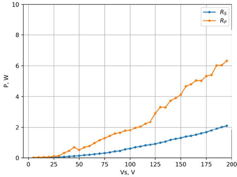
Fig. 2.32.  $R_S$  and  $R_P$  power dissipation dependence on  $V_S$ .
