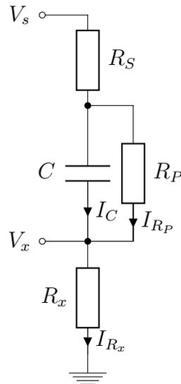
Fig. 2.29. Simplified electrical parameter measurement circuit.
