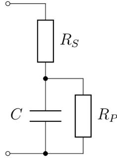
Fig. 2.27.  $LC$  cell equivalent electrical circuit.
