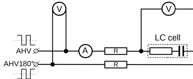
Fig. 2.11. Experimental setup for *SmA LC* cell current limitation and measurements.
