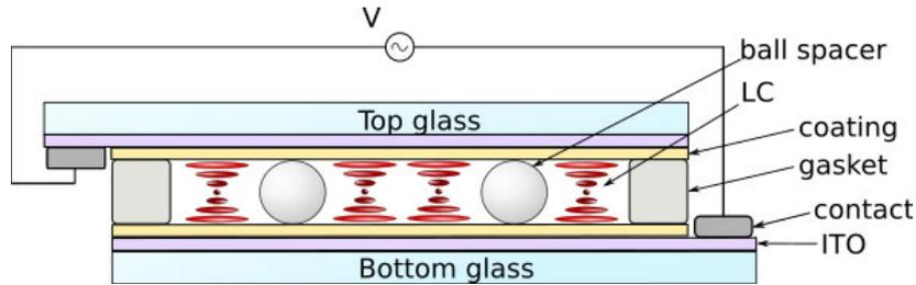
Fig. 2.5. Schematic picture of  $LC$  cell: cross-section [15].
