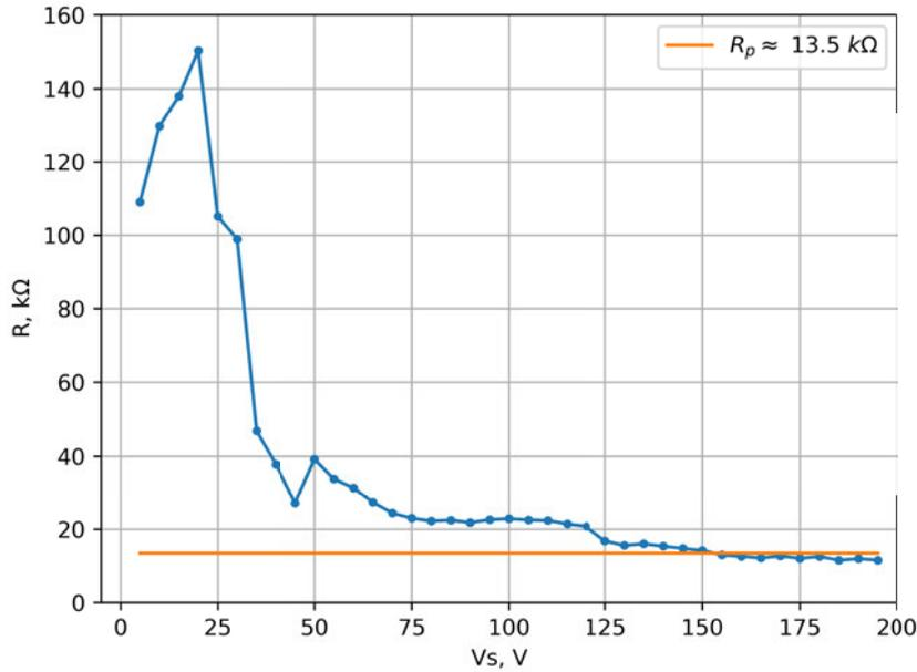
Fig. 2.31. Equivalent parallel resistance  $R_P$  dependence on  $V_S$ .
