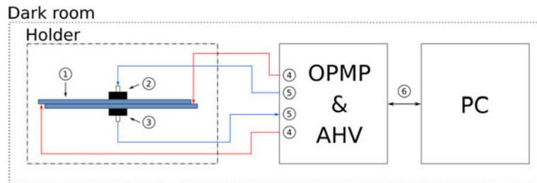
Fig. 2.6. Graphical representation of *SmA LC* cell testing setup.
