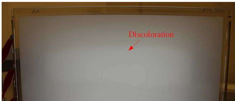
Fig. 2.22. Discoloured pixels, active area of *SmA LC* cell in light scattering state. Additional background (behind the *LC* cell) lightning was used for better visual defect identification.
