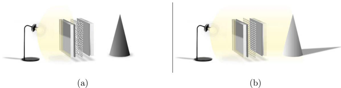
Fig. 2.1. (a) — When off, particles are scattered creating opacity for privacy, shading, solar control, or video projection; (b) — when on, particles align, creating transparency for an open atmosphere and natural light [7].
