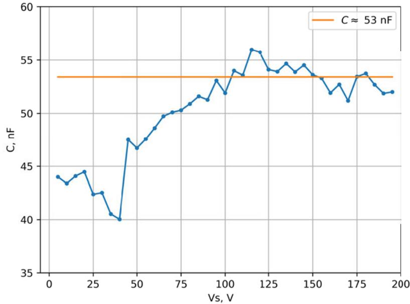
Fig. 2.30. *LC* cell capacitance  $C$  dependence on  $V_S$ .
