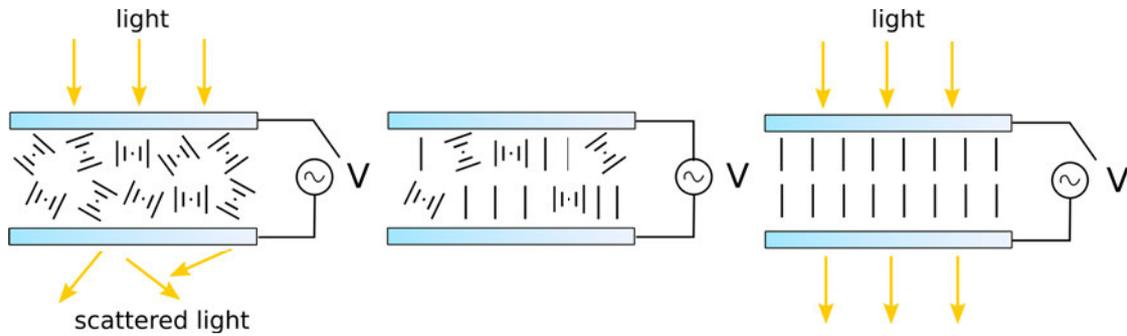
Fig. 2.2. Bistable *SmA* LC cell switching sequence: from the left — light scattering state (electric field is not applied); LC switching in progress (electric field is applied); and light transmittance state (LC cell is fully switched from one state to the other) [10].
