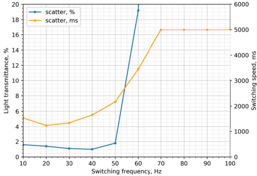
Fig. 2.9. Switching speed (orange) and light transmittance (blue) at different switching frequencies during transition to scattering state.
