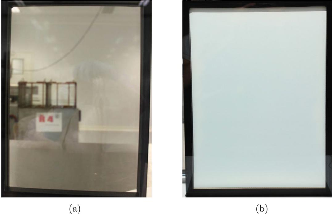
Fig. 2.26. *SmA* LC cell after temperature treatment: (a) — LC cell looks clear due to the LCs, high viscosity (viscosity changes based on LCs temperature), (b) — LC cell after 100+ testing cycles, no visual and functional defects were found.
