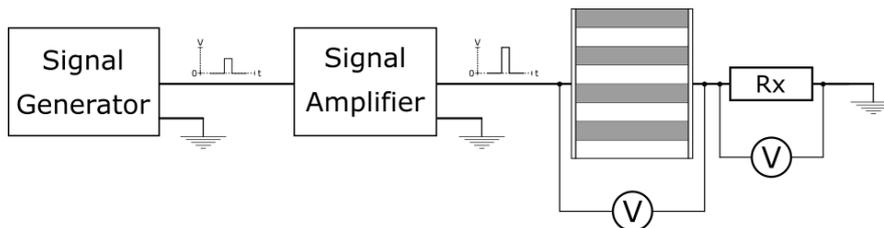
Fig. 2.24. Simplified functional schematic of electrical parameter measurement setup, where waveform generator generates sine wave, sawtooth or other custom signal, signal amplifier amplifies switching signal from 100 V up to  $\pm 200$  V and outputs it to textitSmA LC cell and additional Rx resistance.
