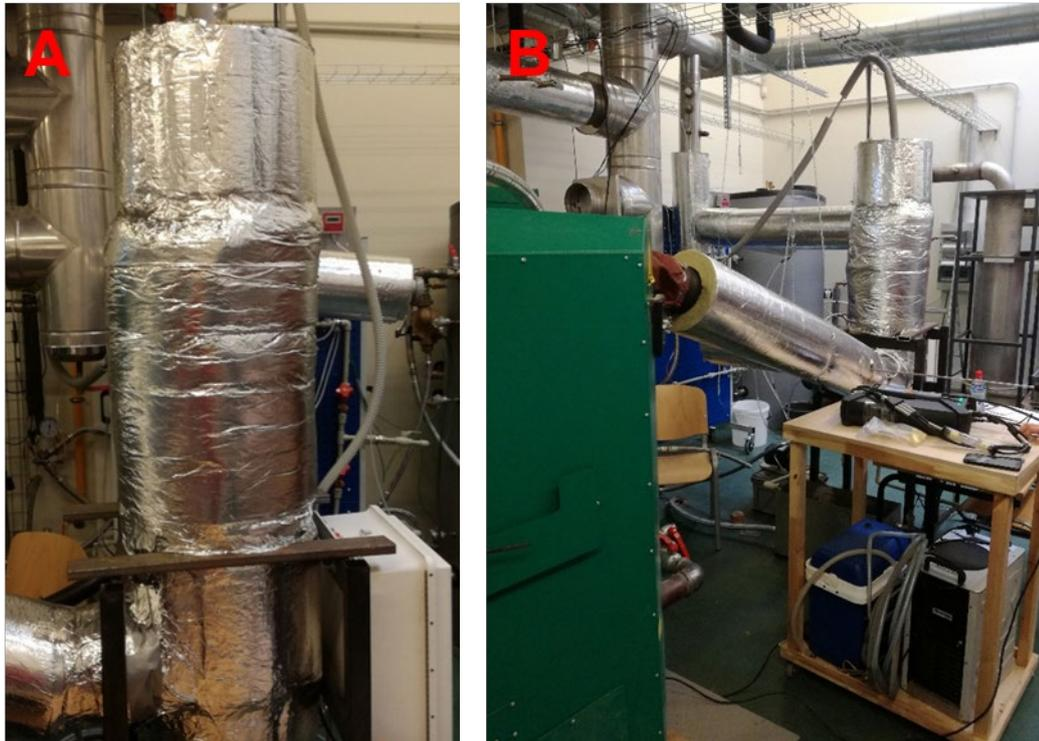
Fig. 2.2. The fog unit in the experimental stand:
