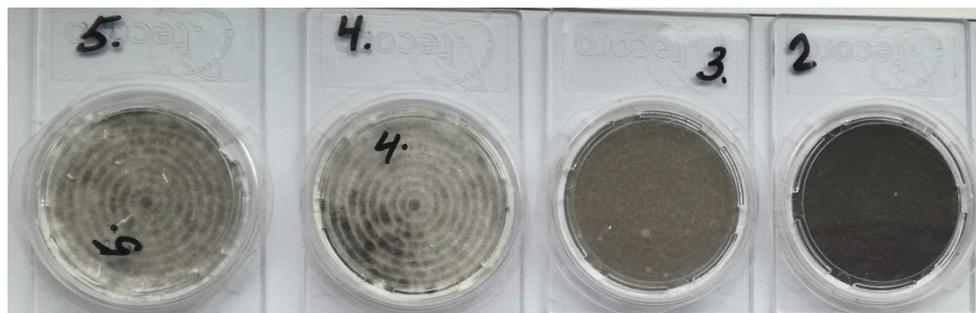
Fig. 2.4. Filters with different particulate matter concentrations
