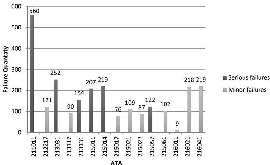
Fig. 6.1. Number of failures of air conditioning system elements during the study period.
