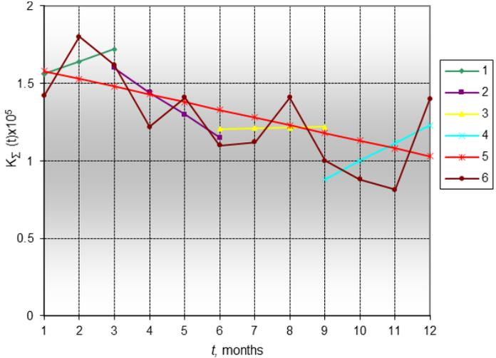
Fig. 6.5. Changes in the number of air conditioning system failures after maintenance periods.
