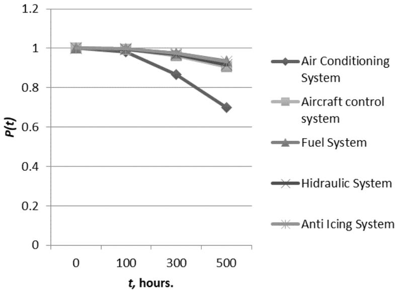
Fig. 6.4. Probability of fail-safe operation of AVRO-RJ70 functional systems.
