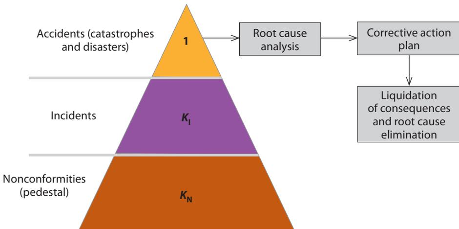
Fig. 1.3. Principle of the reactive management method
