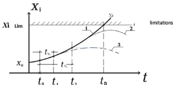
Fig. 5.2. Curve 1 – the curve of the parameter  $X_i$  change at the failure effect; Curves 2 and 3 – parameter change when the pilot (autopilot) reacts and corrects the situation (reaction of the aircraft at different times).
