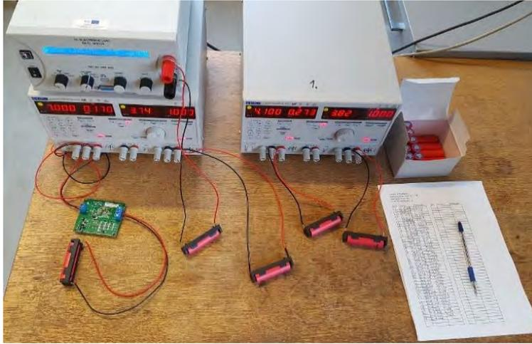
Fig. 4.4. Capacity measurement test equipment.
