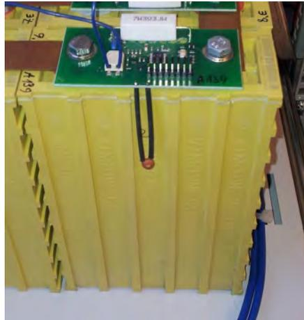
Fig. 6.14. Cell module 3 installed on a 40 Ah LFP cell.
