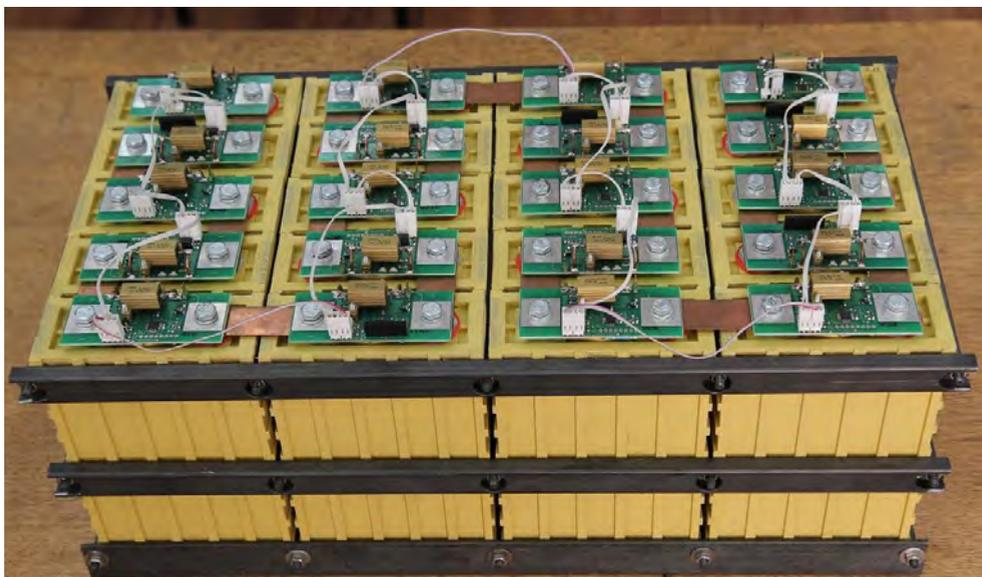
Fig. 6.19. 20-cell LFP battery pack with cell modules 2.
