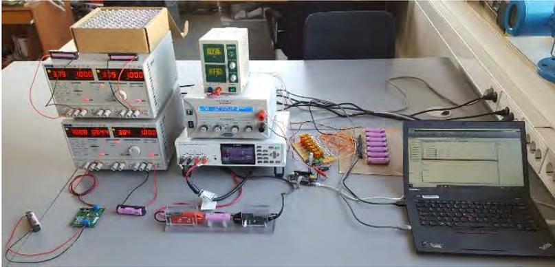
Fig. 4.9. Impedance measurement setup. From left: laboratory power supplies, electronic load, impedance meter, cell switching board, PC for control and measurement storage.
