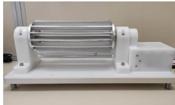
Fig. 2. Rotating drum collector
