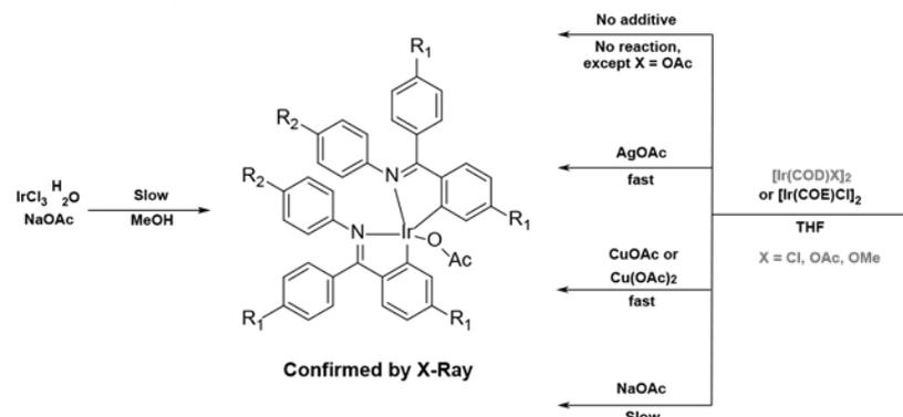
**Figure 1.** Synthesis of bis-cyclometallated Iridium catalyst.
