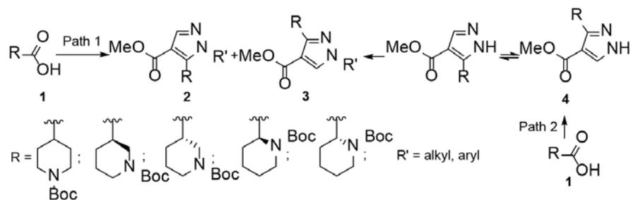
**Scheme 1.** Synthesis of 3(5)-(N-Boc-piperidinyl)-1*H*-pyrazole-4-carboxylate derivatives
