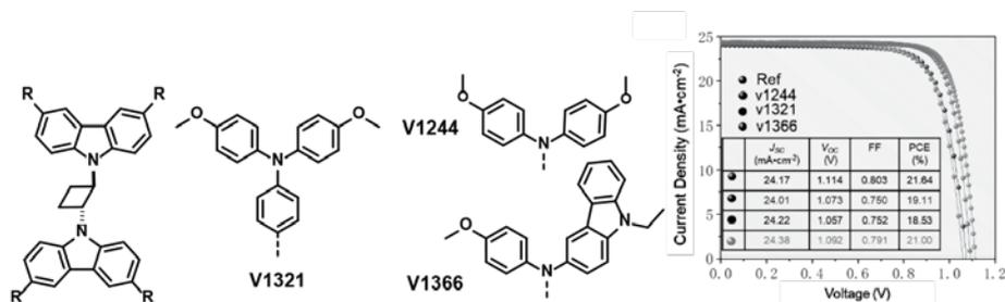
**Figure 1.** J-V curves (reverse-scan) of the PSCs based on **V1244**, **V1321**, and **V1366** as HTMs and spiro-OMeTAD as the reference.
