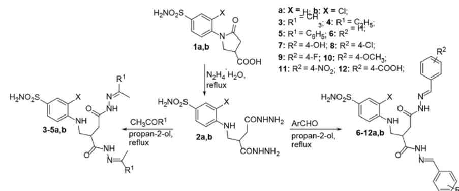
Fig. 1. Synthesis of benzenesulfonamide-bearing dihydrazones
