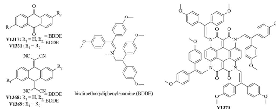
**Fig. 1.** Structures of anthraquinone-based semiconductors.
