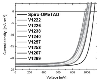
**Figure 1.** *J-V curves of the most efficient solar cells containing Spiro-OMeTAD and new HTMs.*
