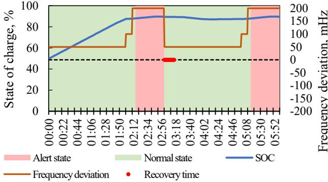
Figure 4. Simulated frequency deviation and LER SOC evolution
