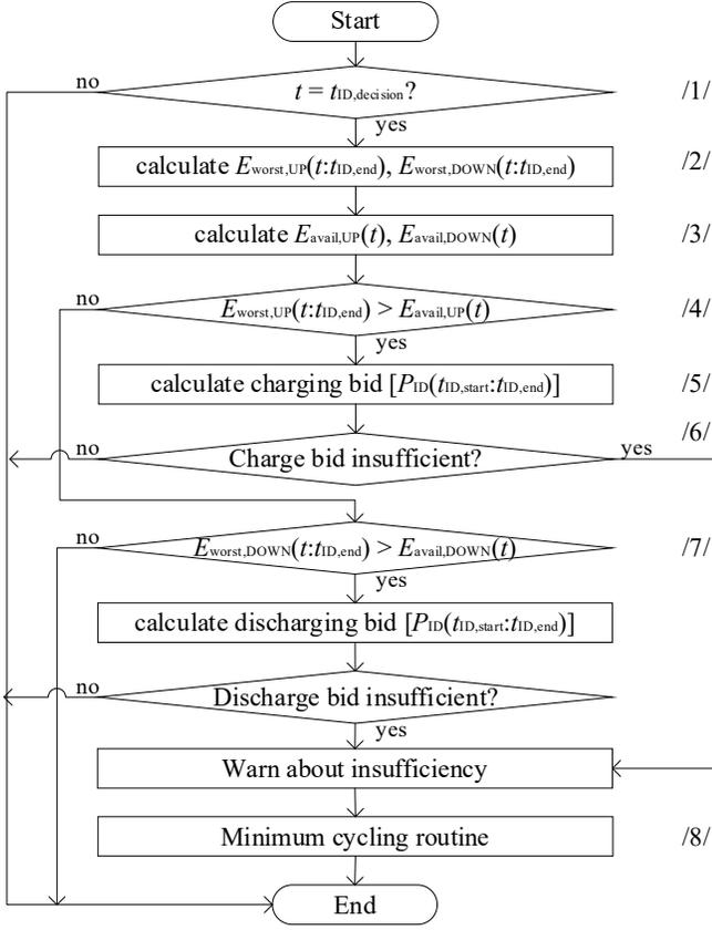
Figure 2. Main steps of the energy recovery algorithm
