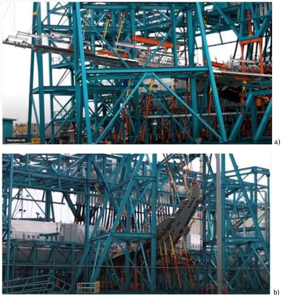
2.2.13. Figure. Facility for breaking testing of Boeing 787 aircraft wing [50]
