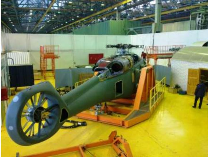
7.5.8. Figure. Fuselage assembly in a removable module
