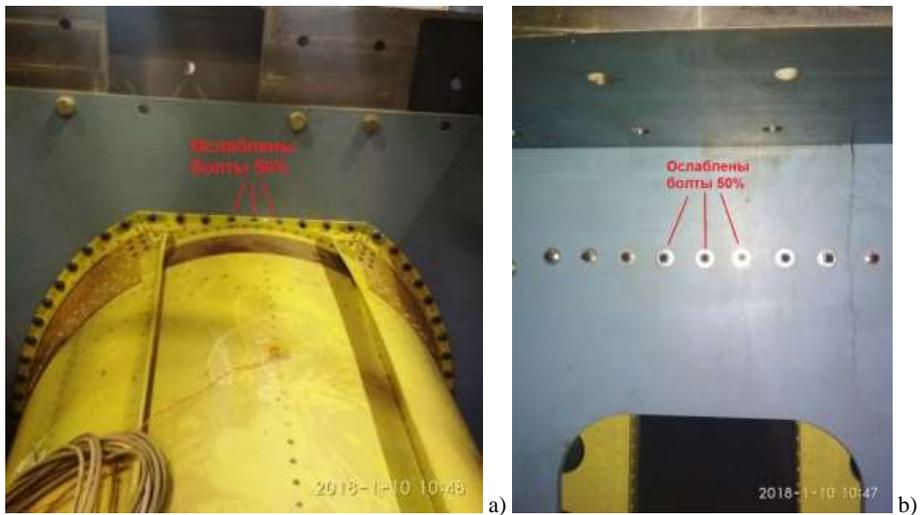
5.6. Figure .The place of easing of the tightening of bolts in the flange connection of the tail boom and fuselage. a) view of the direction of flight; b) view versus flight
