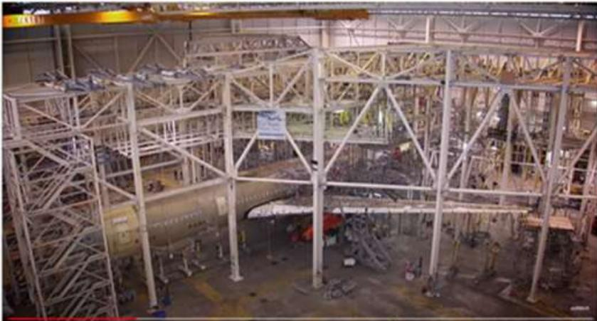
2.2.4. Figure. Facility for full-scale static tests of an aircraft [51]
