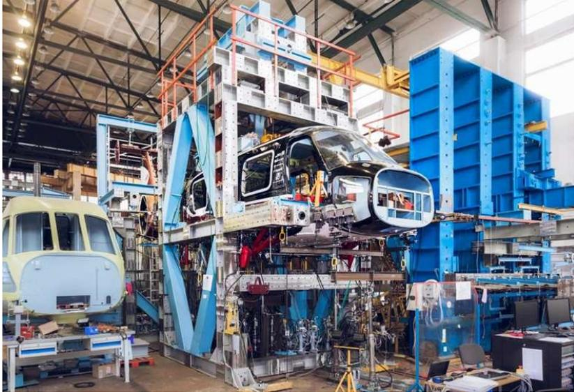
2.2.5. Figure. Facility for full-scale static tests of a helicopter [55]
