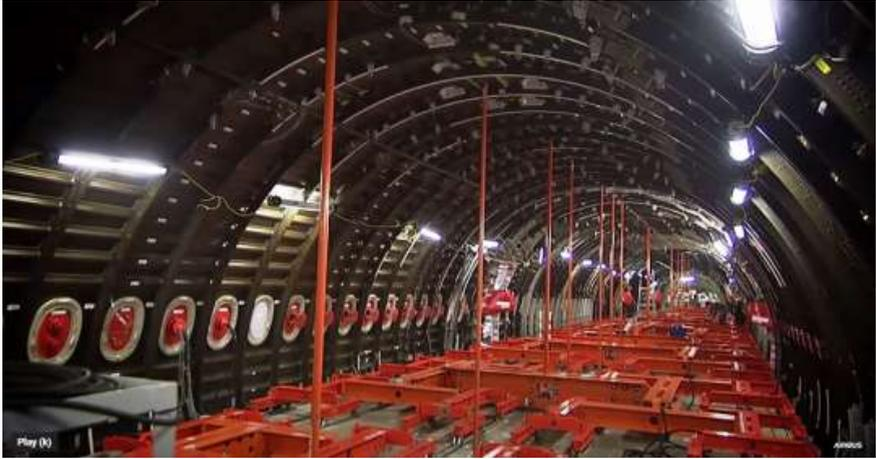
2.2.9. Figure. Testing of the aircraft passenger cabin floor [51]
