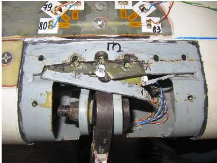
2.3.5. Figure. Destruction of fuselage skin made of composite material [61]
