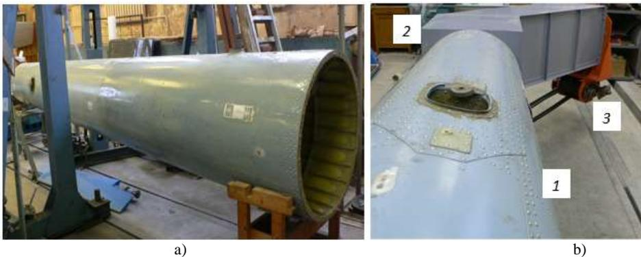
5.1. Figure. General view of the helicopter Mi-8 tail beam (a) and the test setup for dynamic loading (b), 1- the tail beam, 2- imitator of the tail rotor beam, 3 – the eccentric shaker.
