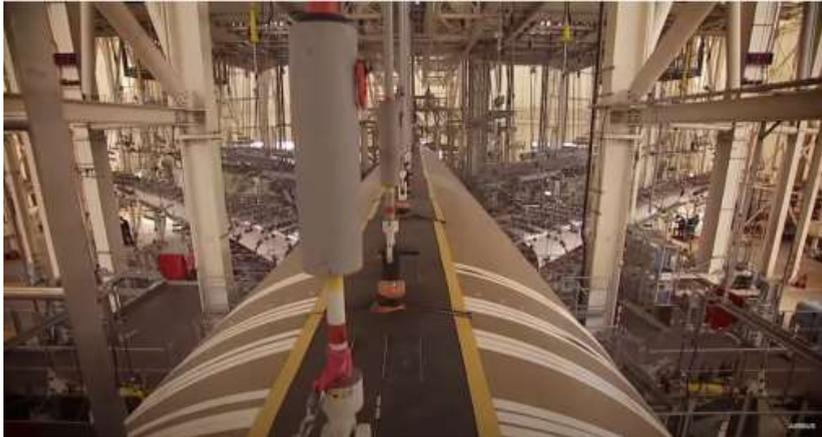
2.2.3. Figure. Facility for full-scale static tests of A-350 aircraft [51]
