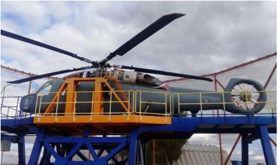
7.5.9. Figure. Helicopter on a power frame
