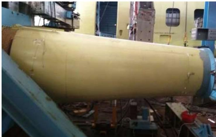
5.3. Figure. The tail boom of the Ka-62 helicopter on the test bench
