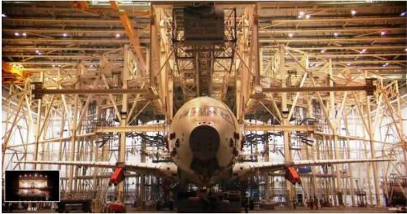
2.2.2. Figure. Facility for full-scale static tests of A-380 aircraft [51]
