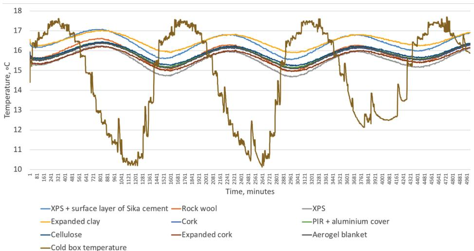
Fig. 2.7. Temperature changes between the masonry and the thermal insulation material in the dynamic test.
