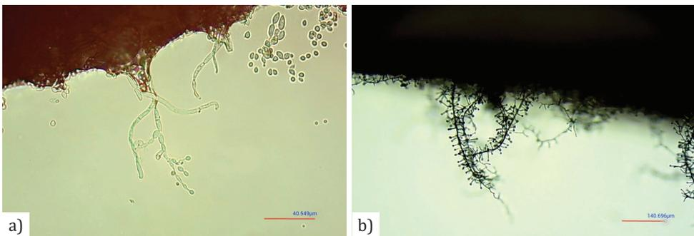
Fig. 2.12. Mould formation on samples at 100 % relative humidity: a) *Cladosporium* on the sample surface without lime; b) *Trichoderma viride* on the surface of the treated sample.
