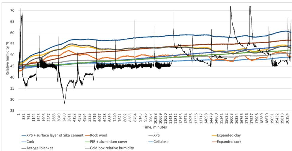
Fig. 2.10. Wind-driven rain test results for nine thermal insulation systems.
