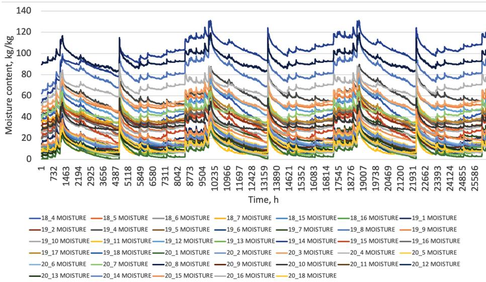
Fig. 2.2. Masonry moisture content for all simulated wall types.
