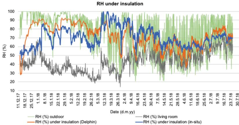
Fig. 2.14. Measured and simulated relative moisture changes in the room and under the insulation.
