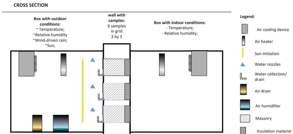
Fig. 1.2. Climate chamber's schematic representation.
