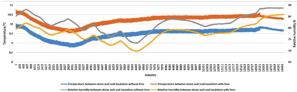
Fig. 2.13. Relative humidity and temperature under varying conditions between the stone wall and needle insulation with and without lime.
