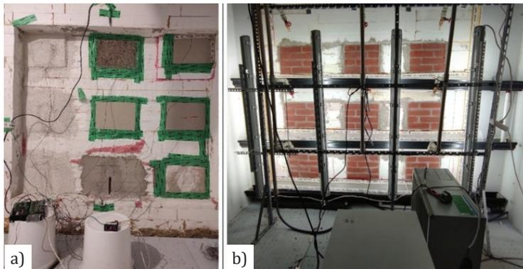
Fig. 1.3. Test wall With nine masonry wallsamples a) from warm side b) from the cold side.
