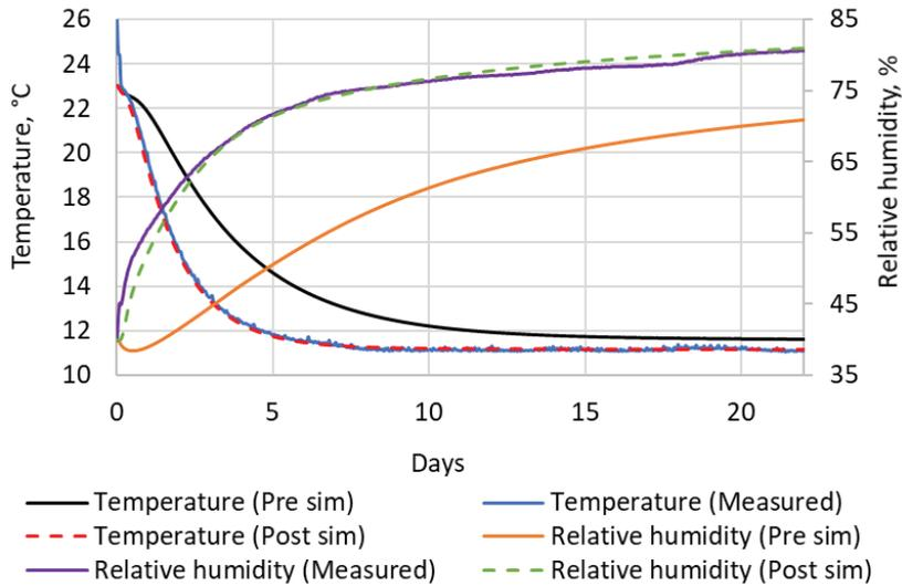
Fig. 2.5. Temperature and relative moisture behaviour between the masonry and fibreboard without steam barriers: simulation before and after the experiment and measurement results.
