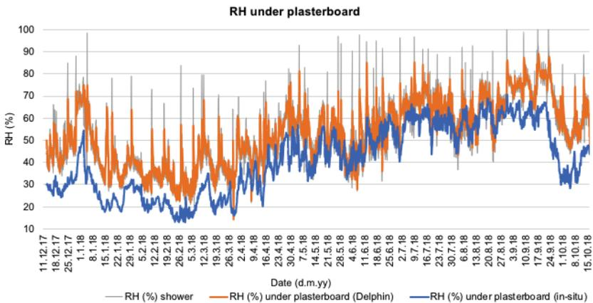
Fig. 2.15. Changes of relative moisture in the room and under thermal insulation and simulated relative moisture values in the bathroom.
