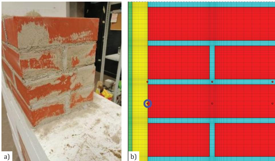
Fig. 1.5. Test wall sample a) in the laboratory and b) in the Delphin model.
