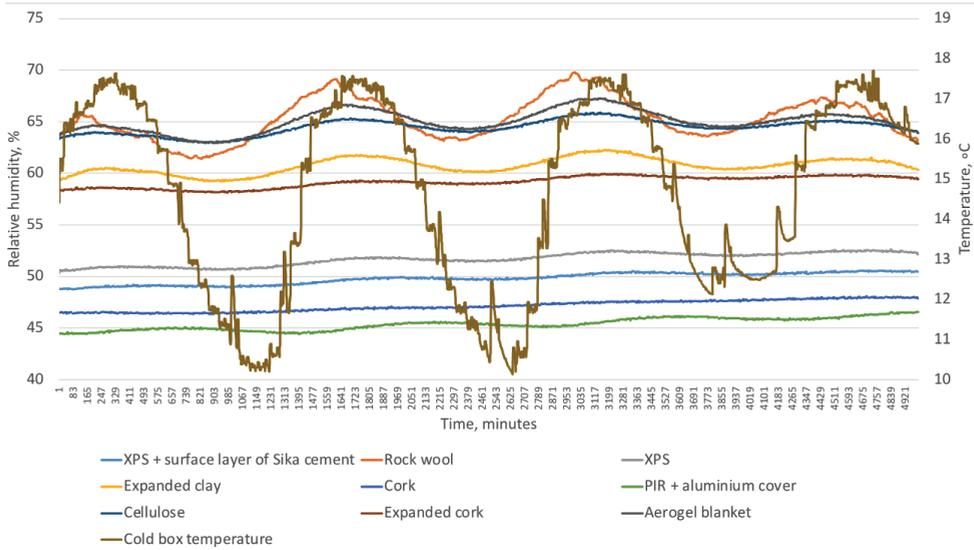
Fig. 2.9. The relative humidity between the thermal insulation and the masonry when the indoor relative humidity is stable and the outdoor temperature fluctuates (dynamic cycle).
