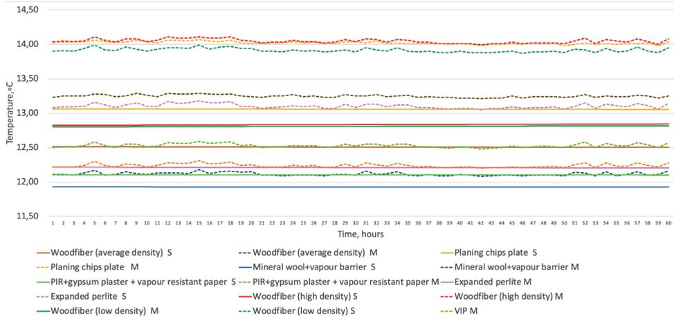
Fig. 2.6. Simulated (S) and measured (M) temperature between the thermal insulation material and the masonry wall in the equilibrium cycle (time period between 245 and 305 minutes).
