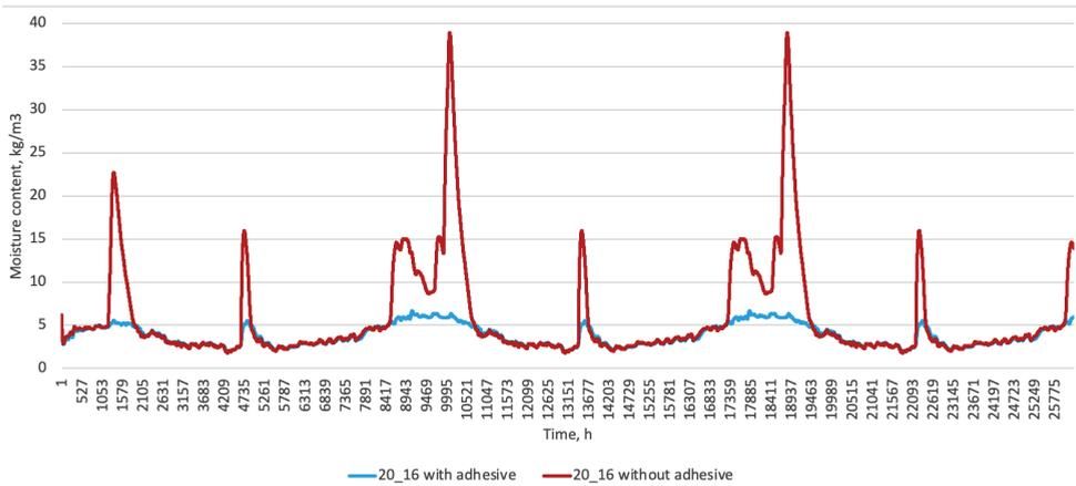
Fig. 2.3. Moisture content of thermal insulation material brick 20\_18 masonry with and without glue.
