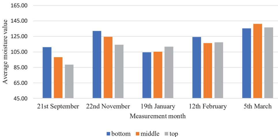
Fig. 2.19. Changes in average values in the upper, middle, and lower parts for dielectric measurements at a depth of 2 cm.
