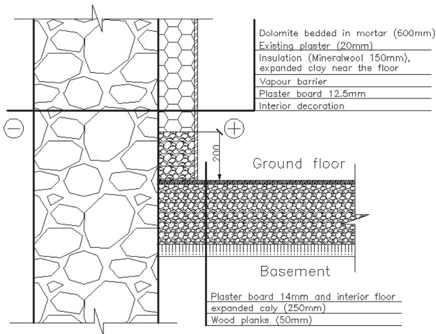
Fig.1.7. Residential rooms – cross section of external walls and floors after the 2015 renovation.
