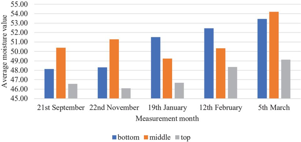
Fig. 2.18. Changes in the average values in the upper, middle, and lower part of the wall for microwave measurements at a depth of 20 cm.
