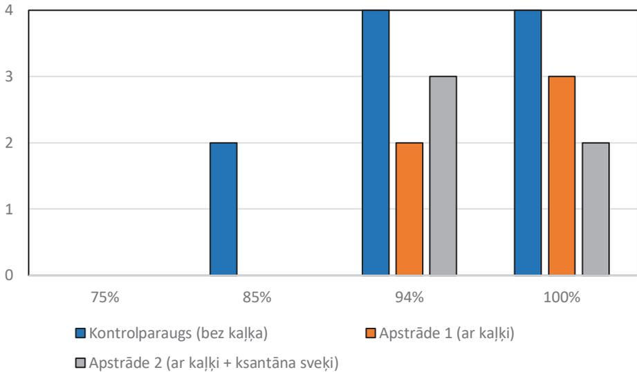
Fig. 2.11. Mould growth on material samples under different relative humidity conditions (blue – control group; orange – with lime; gray – lime + xantan).
