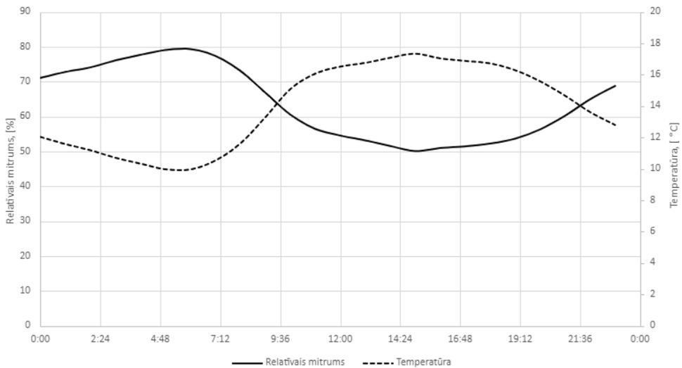
Fig. 1.4. Diurnal climate fluctuations in May selected as the basis for the dynamic test cycle.
