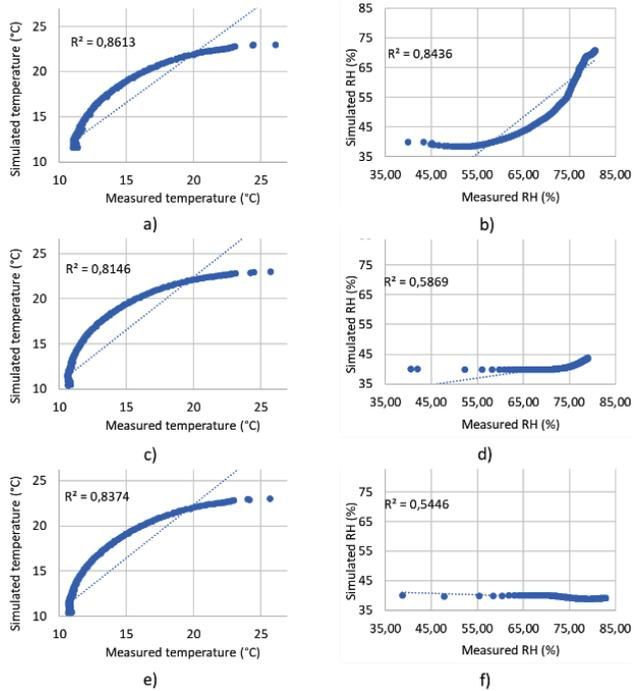
Fig. 2.4. Correlation between the modelled and measured temperatures between the masonry and the insulation layer: a) wood fibre; c) EPS; e) mineral wool) and relative humidity: b) wood fibre; d) EPS; (f) mineral wool).
