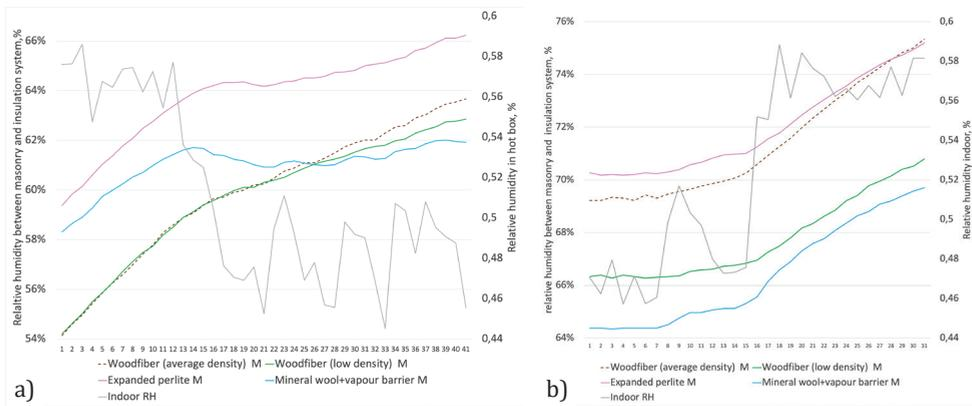
Fig. 2.8. Changes in relative humidity between the masonry and vapour-permeable thermal insulation material when the relative humidity of the room a) decreases and b) increases.
