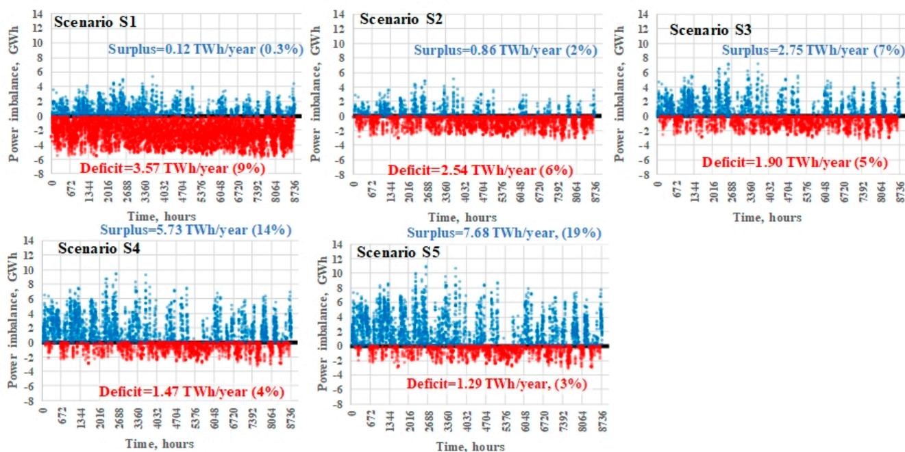
**Figure 8.** The power imbalance of the BPS in 2050, assuming operational interconnections but no HECME power plants. Results of the scenarios S1, S2, S3, S4 and S5 modelling.
