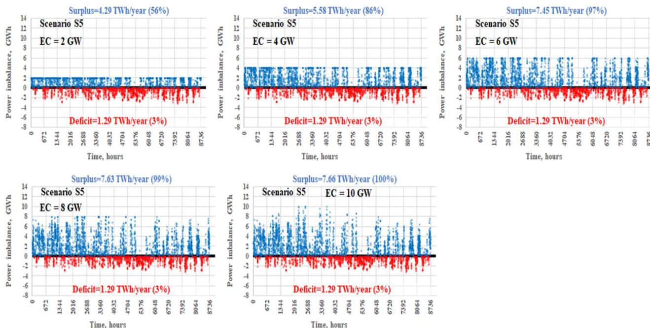
**Figure 16.** Power imbalance in the BPS in S5 that is addressed by the HECME with varying installed capacities of electrolysers (EC). The annual deficit is specified in TWh/year and in percent of total power demand in the BPS. The annual energy consumption by the electrolysers (the surplus) is shown in TWh/year and in percent from the total energy surplus in the BSP.
