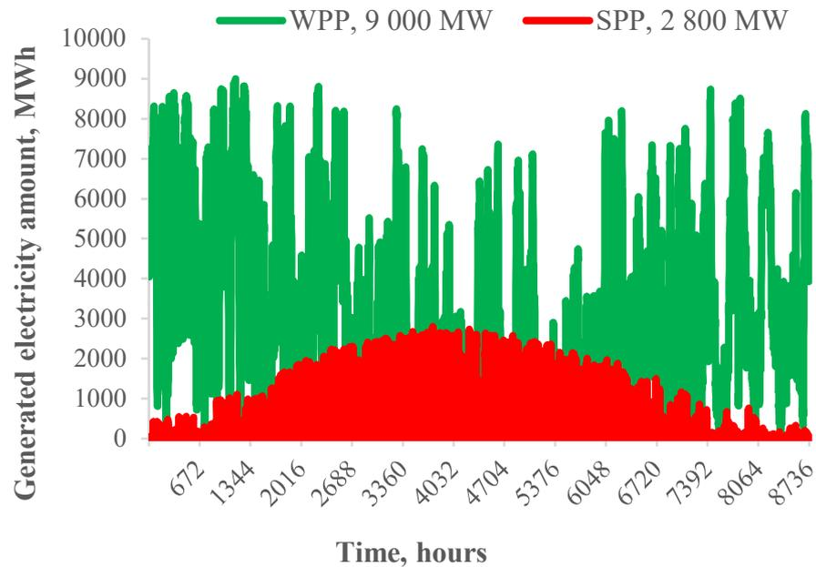
Figure 5. Hourly forecasts of RES-generated energy in the BPS in 2050.
