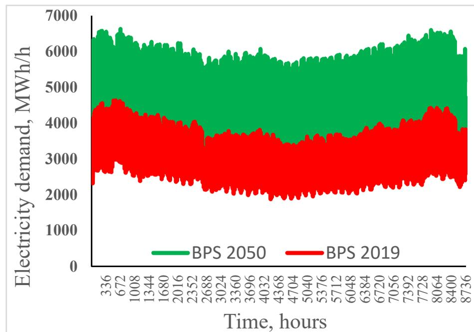
Figure 6. Hourly consumption in the BPS in 2019 (27.56 TWh/year) and in 2050 (39.83 TWh/year).
