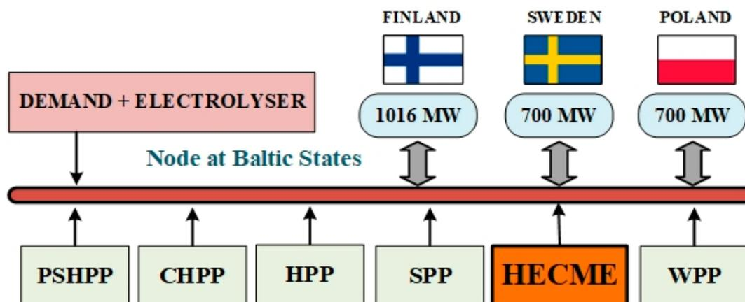
**Figure 2.** The portfolio of the power plants and the interconnections: a pumped storage hydropower plant (PSHPP), a hydropower plant (HPP), small HPPs (sHPP), a solar power plant (SPP), a wind power plant (WPP), a power plant based on hydrogen production, conversion to methane and back to electricity (HECME), a combined heat and power plant (CHPP), electricity loads (Demand) and interconnecting DC and AC power lines between the Baltic States and Finland, Poland, Sweden.
