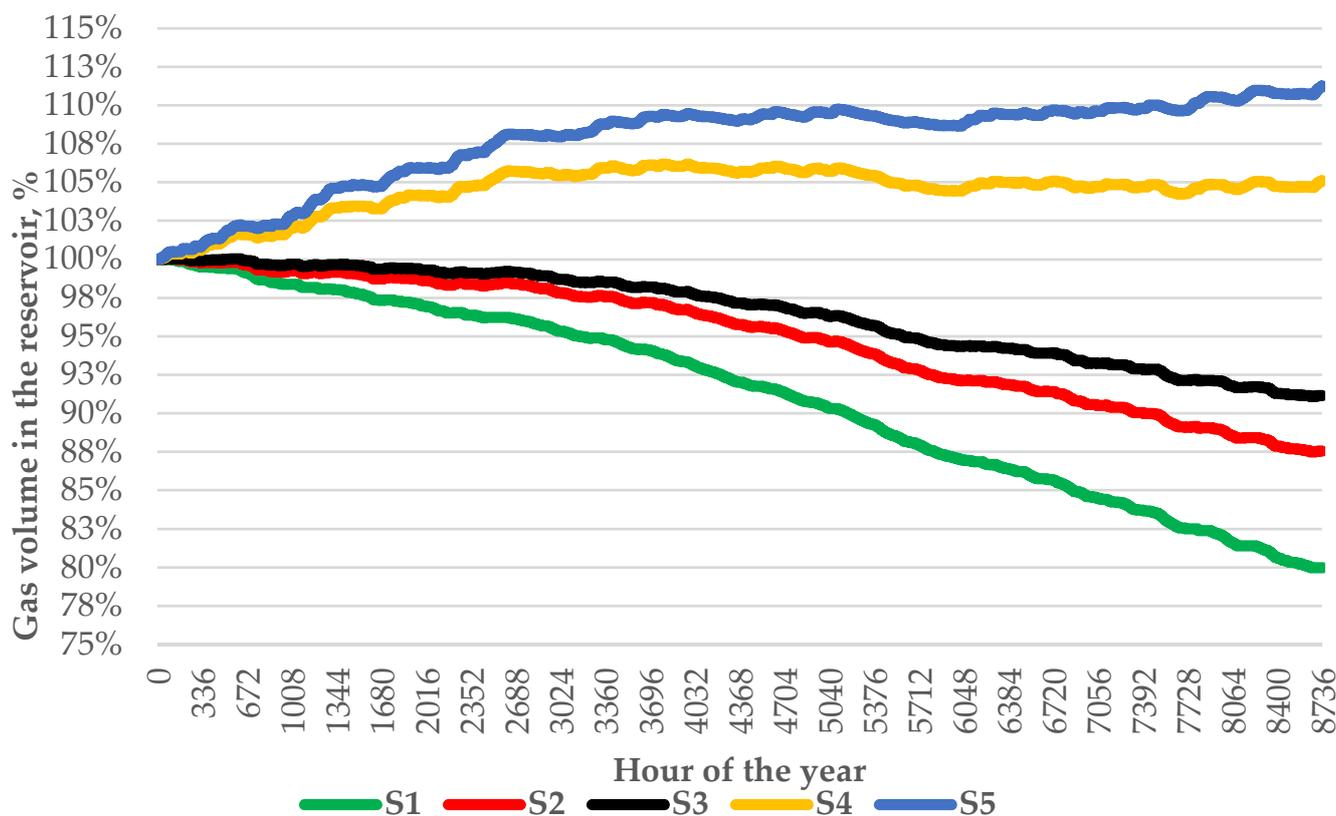
Figure 10. Evolution of gas volume in the reservoir over a year.
