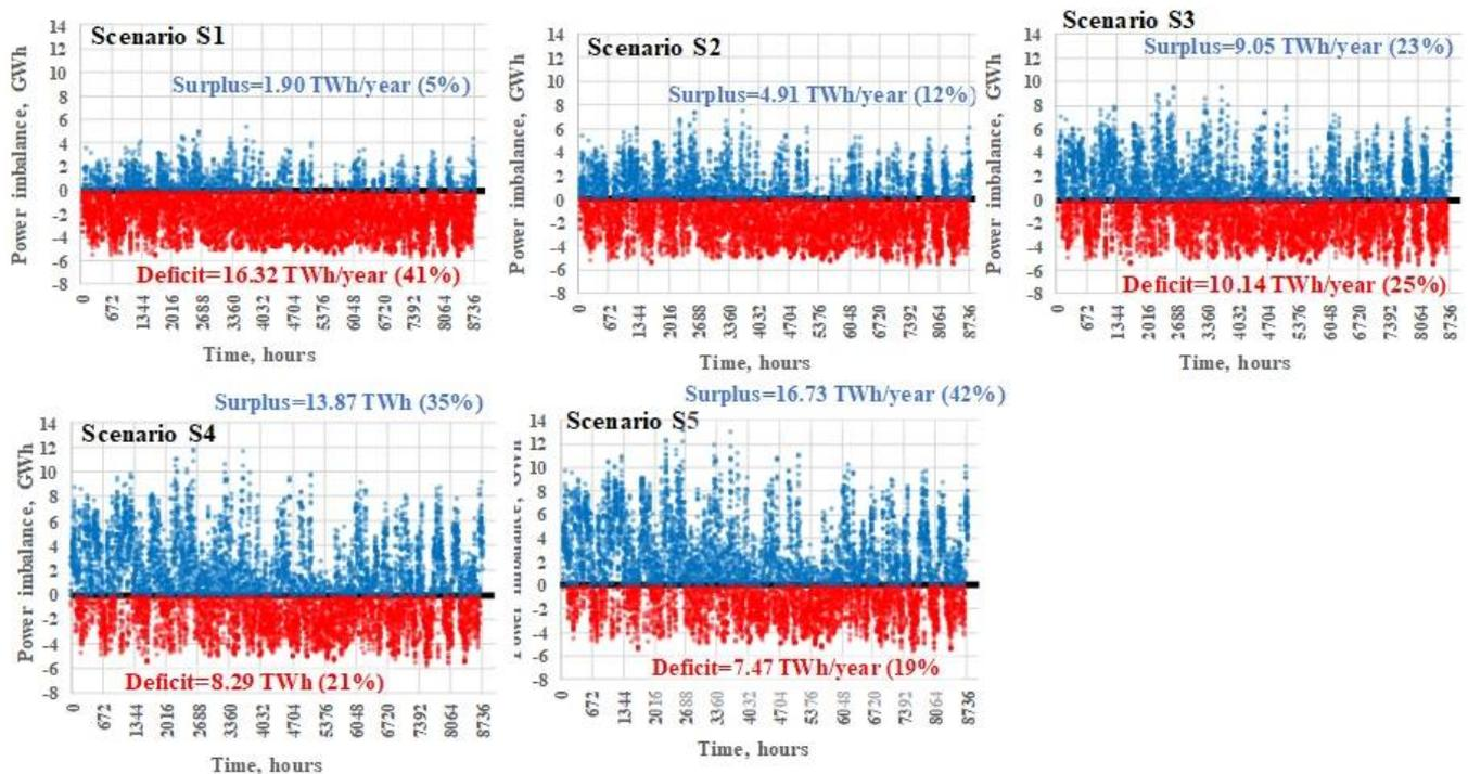
**Figure 7.** The energy balance of BPS 2050 in an islanded mode for scenarios S1, S2, S3, S4 and S5.
