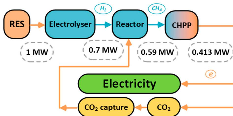
**Figure 1.** Energy conversion and efficiency in a hydrogen energy conversion to methane energy power plant (HECME PP).
