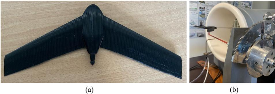
Fig. 6.1. (a) – 3D printed in 10 % scale UAV model; (b) – printed model mounted on the wind-tunnel.
