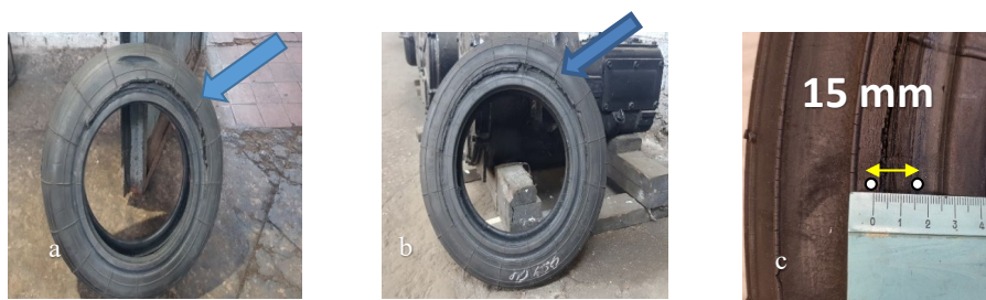
Fig. 3.1. Examples of the side surface disintegration of a rubber- cord coupling: a – sample 1; b – sample 2; c – determining the destruction zone sample 2.
