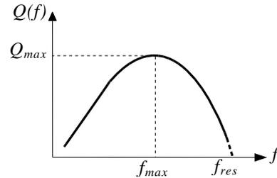
Figure 2. Typical frequency dependence of Q-factor
