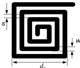
Figure 1. Geometry of a planar spiral inductor [6]
