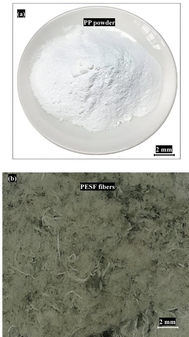
Fig. 2. Materials for fabrication of PP-PESF composites: (a) Pure virgin PP and (b) fibers of PES waste.
