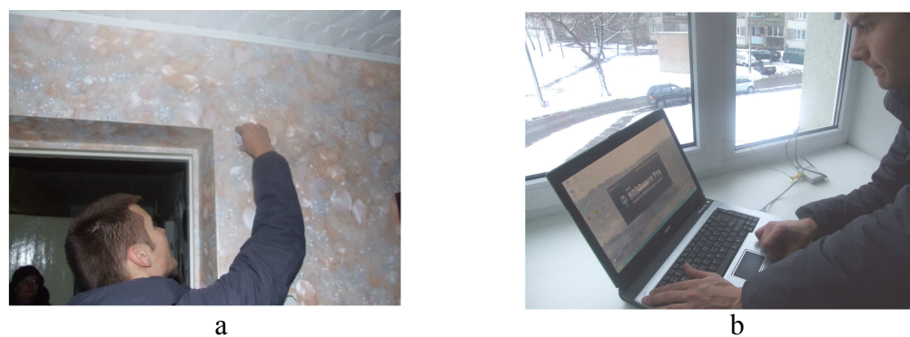
Figure 3. Placing of temperature loggers (a) and data retrieving (b)
