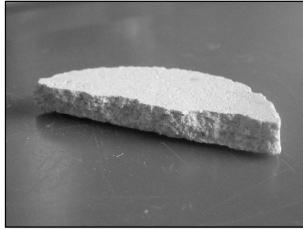
Fig.14: Sample of “sacrificial” plaster (0.6 cm thick)
