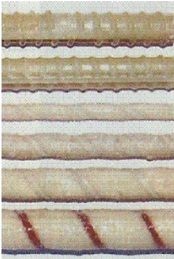
Figure 7. Glass fibre hybrid polymer composite bars (picture from [10])
