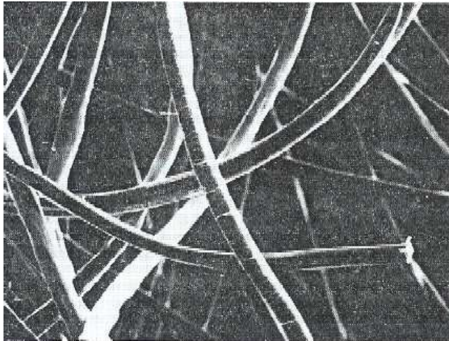
Figure 5. Extruded ordinary polypropylene fibers (picture from [7])
