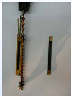
Fig. 2. The picture of sample alone and in the sample holder set up for electric resistance measurements in vapor atmosphere.
