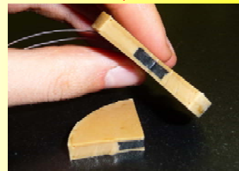
Fig.9 The functional multilayer complete sensing element prototype. The disk shaped active and conductive layers are moulded into isolative polyisoprene shell.
