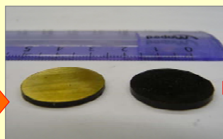
Fig.2 The preliminary test samples with (left side) and without (right side) brass foil electrodes.
