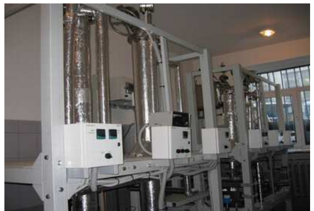
Fig. 6. Pilot plant for obtaining furfural, acetic acid and lignocellulose from wood for bioethanol production
