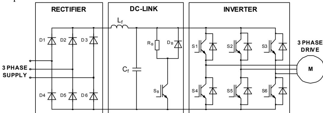
Fig. 2.2. Voltage source inverter schematic diagram
