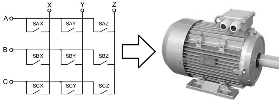
Fig. 2.1. Induction motor integrated drive concept with matrix converter
