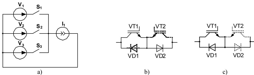
Fig. 2. 16. Equivalent schematic of a) one output phase of MC; b) bi-directional switch during static period; c) bi-directional switch during dynamic period
