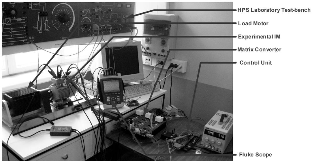
Fig. 2.23. Experimental setup of Induction Motor Drive with Matrix Converter
