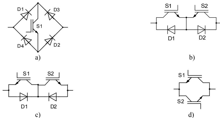
Fig. 2.6. Bi-directional switches a) diode bridge bi-directional switch configuration; b) common emitter configuration c) common collector configuration; d) anti-parallel NPT IGBT configuration
