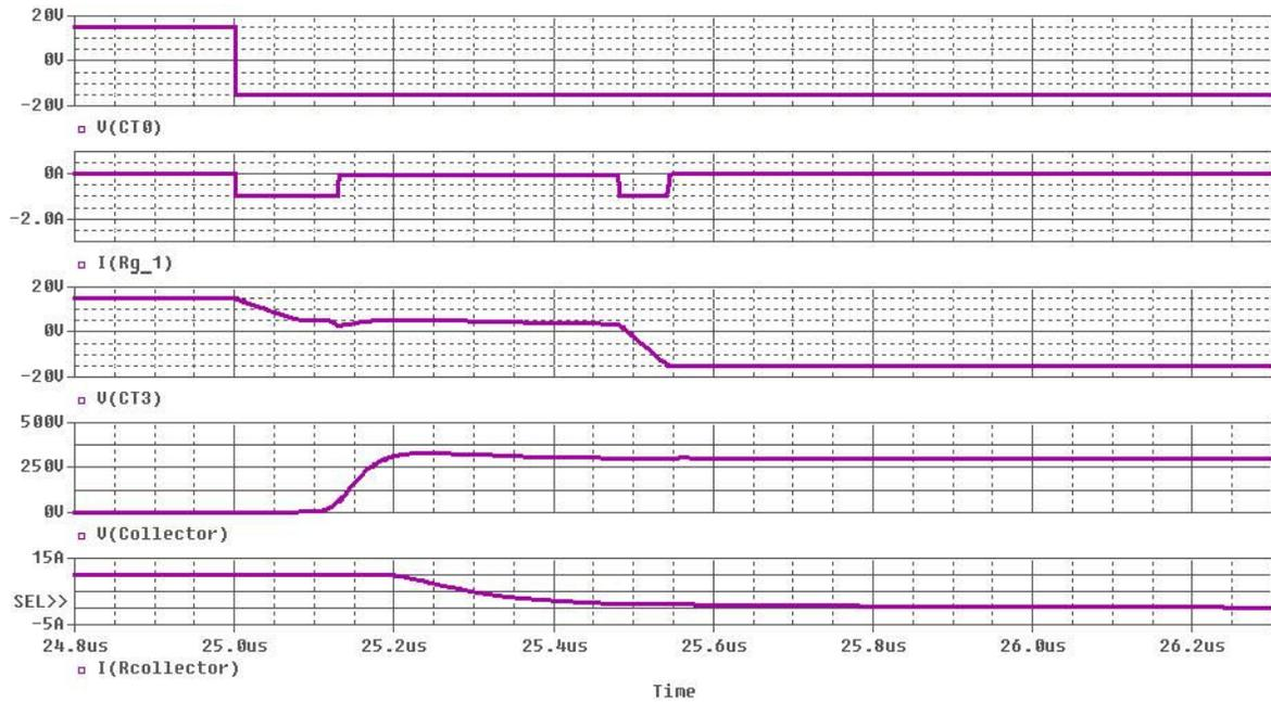
Fig. 2.9. Simulation results of IGBT turn-off with two-level gate current control
