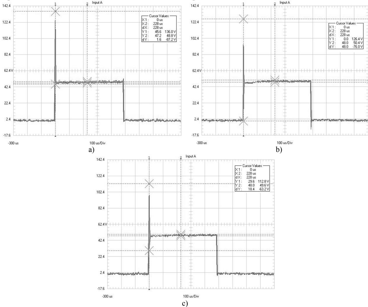
Fig. 2.14. Experimental results of switch commutation: a) without bus bars; with implementation of planar bus bar construction: b) more distant conductors, c) closest conductors
