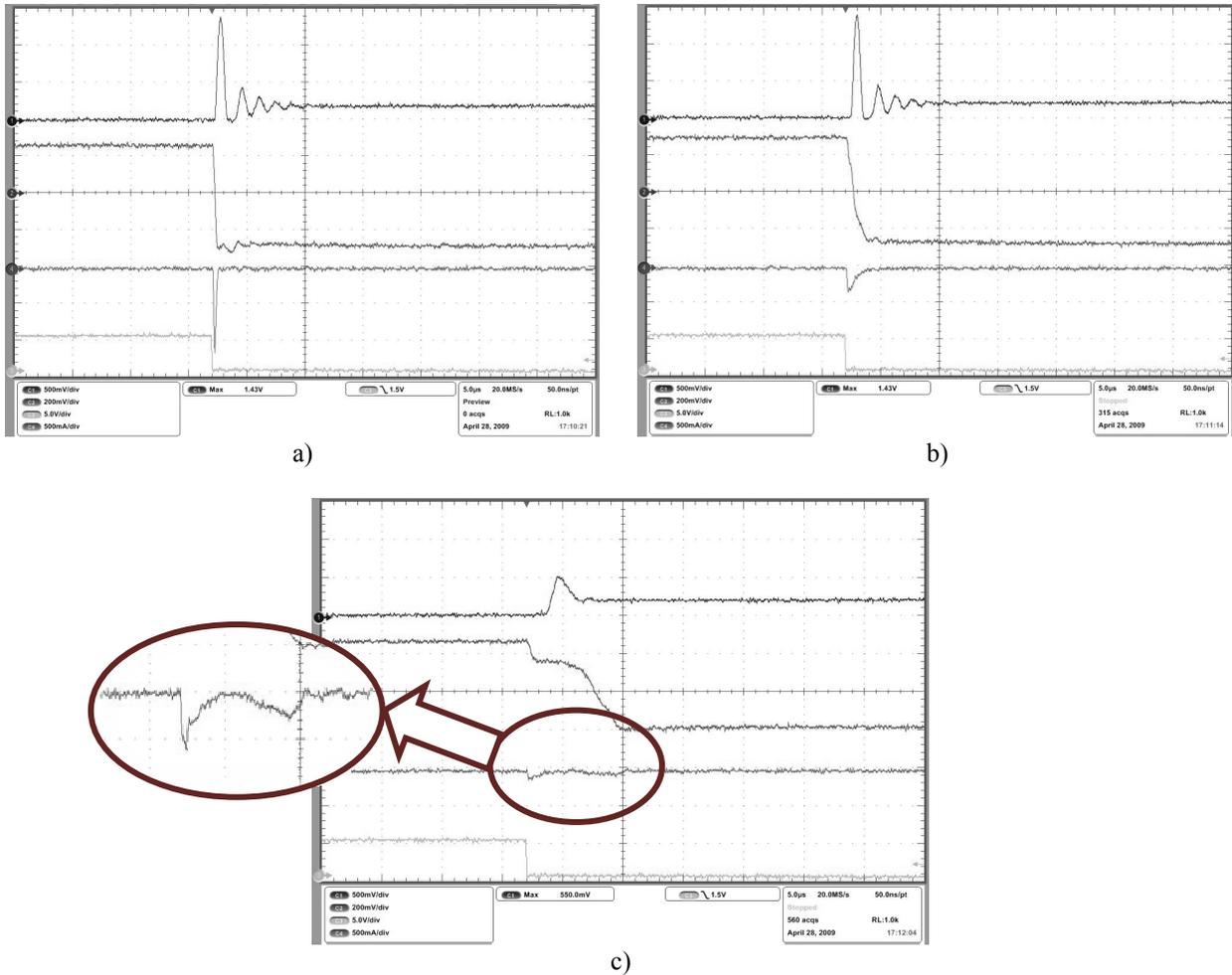
Fig. 2.10. Experimental results of a) passive gate current control commutation at  $R_G = 10\Omega$ ; b) passive gate current control commutation at  $R_G = 50\Omega$ ; c) active two-level gate current control commutation
