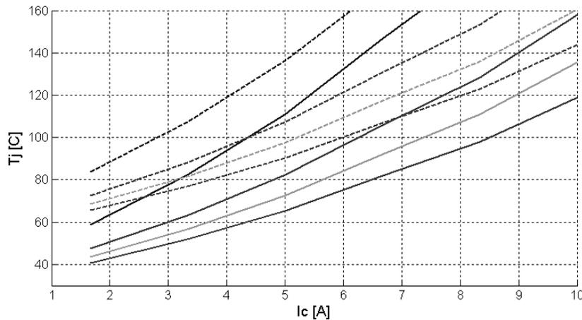
Fig. 2.19. Junction temperature as function of collector current at different cooling conditions; From top: natural convection, forced cooling at 1m/s, forced cooling at 2m/s, forced cooling at 5m/s; Solid line at ambient temperature 25°C, dashed line at ambient temperature 50°C
