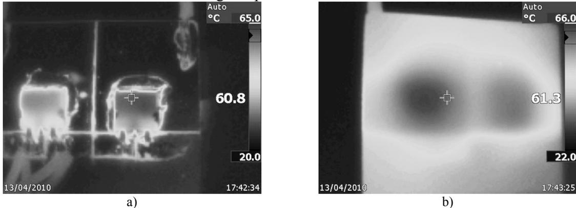
Fig. 2.21. Temperature of a) bi-directional switch at 1.4 A at commutation frequency 13 kHz; b) back side of PCB
