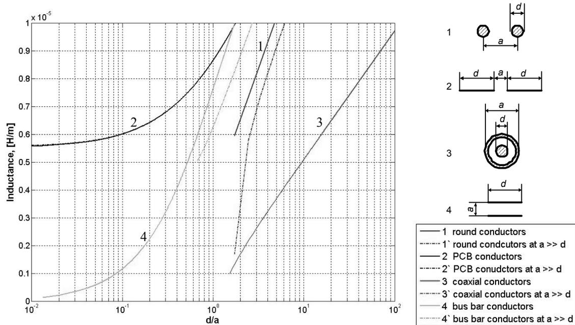
Fig. 2.11. Theoretical inductance characteristics of different conductor shapes
