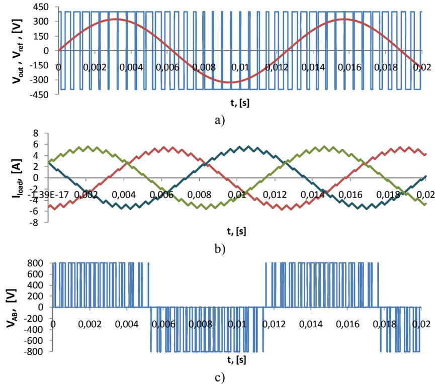
Fig. 2.3. VSI a) bipolar phase voltage (blue – SPWM, red – reference); b) three phase current; c) output line-to-line voltage
