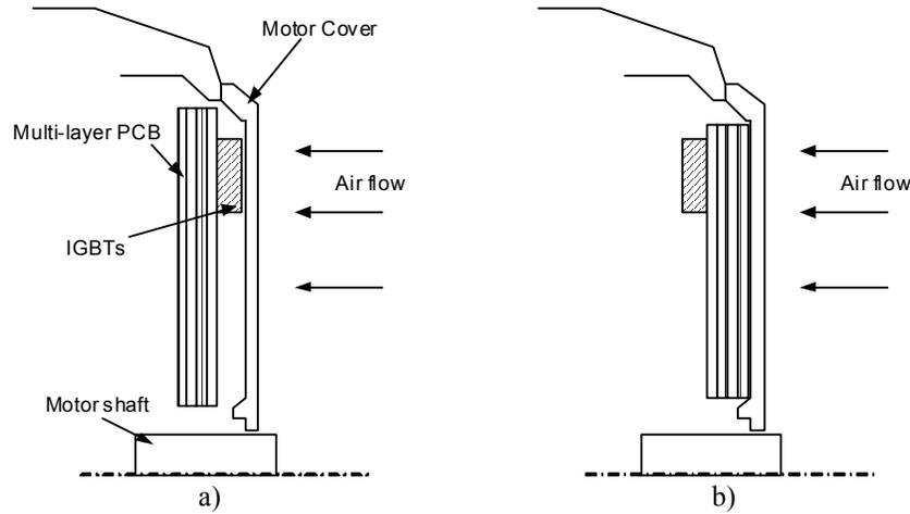
Fig. 2.18. Power board placement on the cooled area of induction motor a) transistor-to-cover, b) bus bar-to-cover
