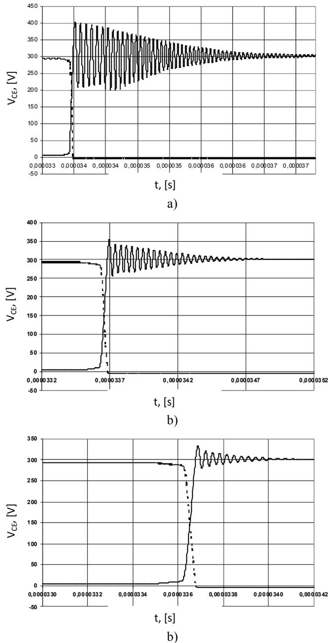
Fig. 2.12. Matrix converter commutation overvoltage a) at 500nH; b) at 100nH; c) at 50nH; solid line – collector-emitter voltage of VT\_AX, dashed line – collector-emitter voltage of VT\_CX
