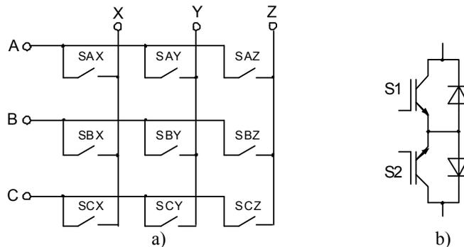
Fig. 2.4. Matrix Converter a) three-phase to three-phase topology, b) typical bi-directional switch
