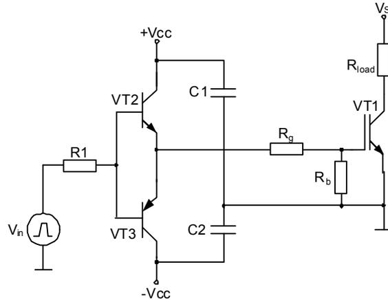
Fig. 2.7. Double-fed Half-Bridge topology
