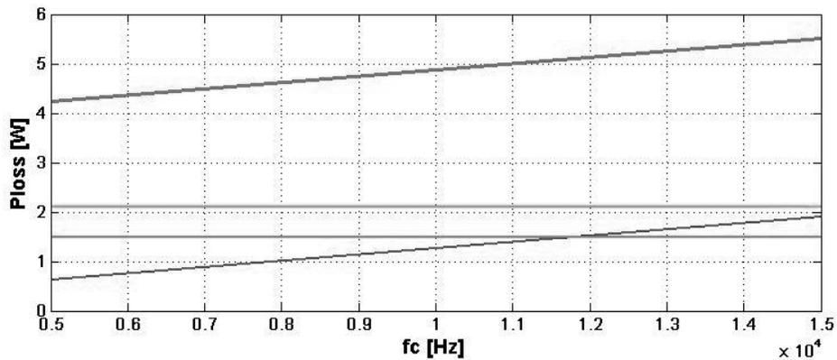
Fig. 2.17. Power losses of Matrix Converter;
