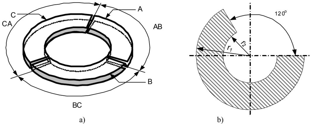
Fig. 2.15. Planar disc bus bar configuration a) 3D layout; b) top view of one conductor
