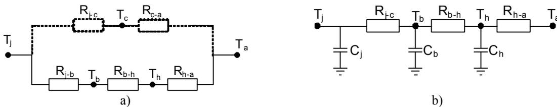
Fig. 2.18. Thermal equivalent circuits for a) steady state heat flow; b) transient operation
