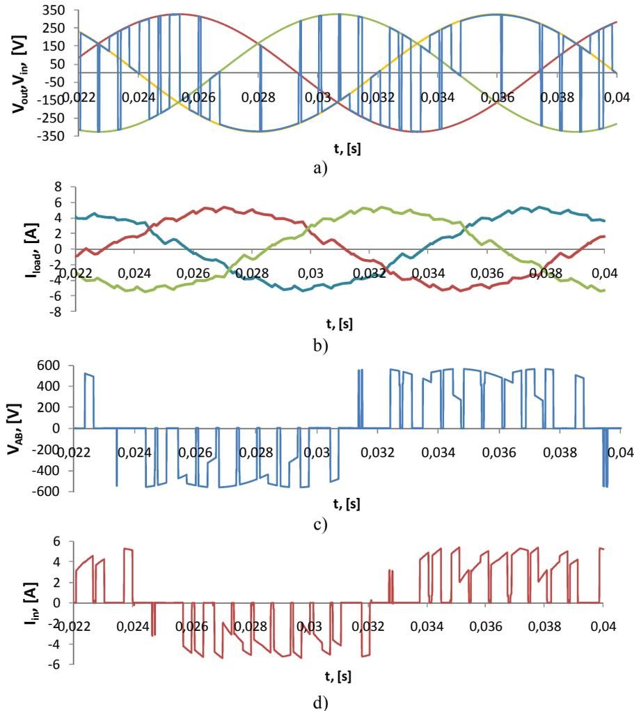
Fig. 2.5. Matrix converter a) output PWM phase voltage; b) three phase load current; c) output PWM line-to-line voltage; d) input current
