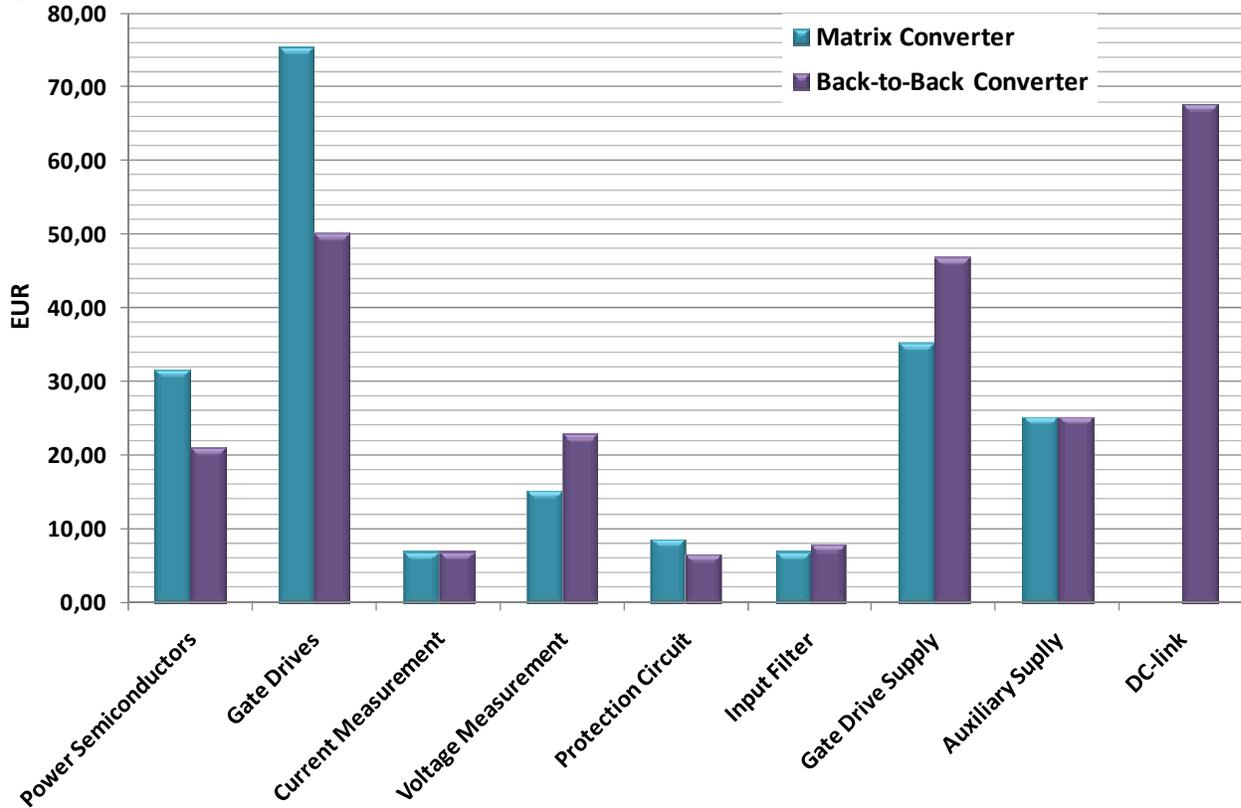
Fig. 3.1. Matrix Converter and Back-to-Back Converter laboratory prototype expense comparison
