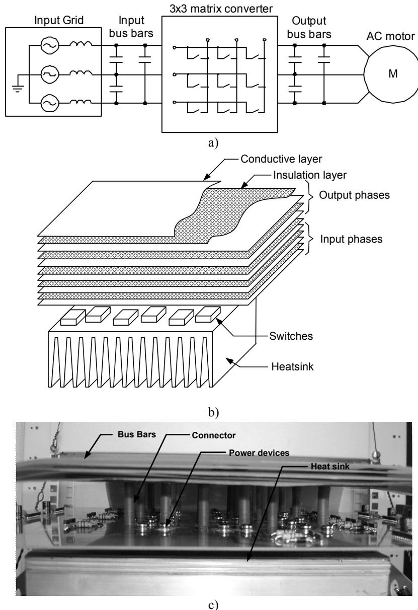
Fig. 2.13. Planar bus bar system for 3x3 matrix a) principal schematic, b) sketch drawing, c) laboratory prototype
