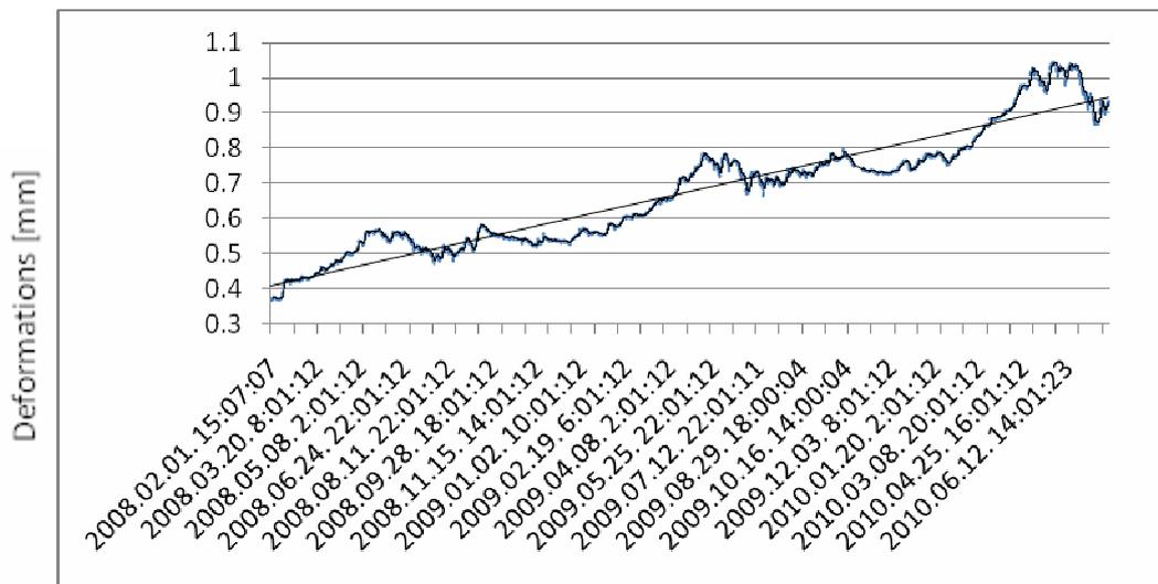
Picture 10. Sensor 5740 is placed on the arch rib along axis “2”, between axes “C” and “D” on the hall side, at the bottom of the arch rib. The crack does not show direct displacement of the arch rib external hinge, however together with sensor 5739 shows separation of the wedge-shaped brick cladding made during the earlier reconstruction of the original arch rib. The wedge closing makes the arch rib more flat however the crack does not ensure joint action of the original arch and the sealing.
