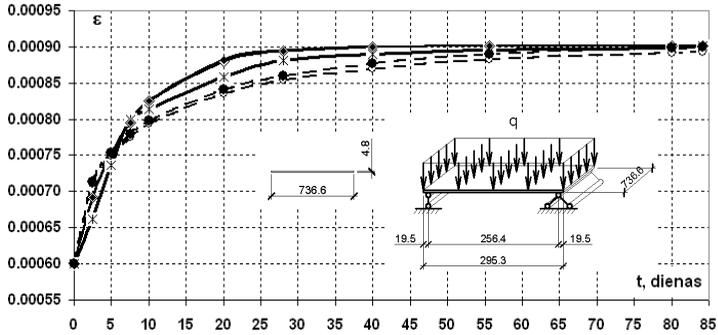
Fig 4.3. Loading scheme, cross-section and creep curves of plywood plate, if load  $q=4.323\text{kN/cm}^2$ . Decoding of patterns see in fig.4.2.
