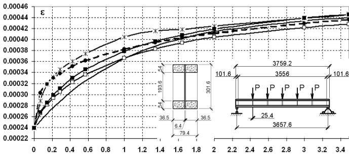
Fig.4.4. Loading scheme, cross-section and creep curves of composite wood I-beam-1, if load  $P=1.089\text{ kN}$ . Decoding of patterns see in fig.4.1.
