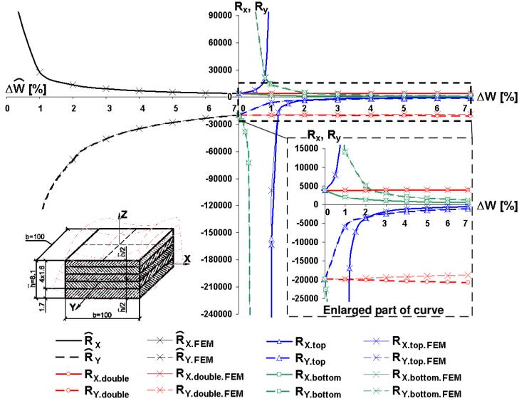
Fig 2.2. Change in bending radiuses  $R_x$  and  $R_y$  in dependence of the material moisture changes for the concave-convex sheet (on the left side of the graph) and for the strengthened elements (on the right side of the graph) if the thickness of the reinforcement is 3.15 mm.
