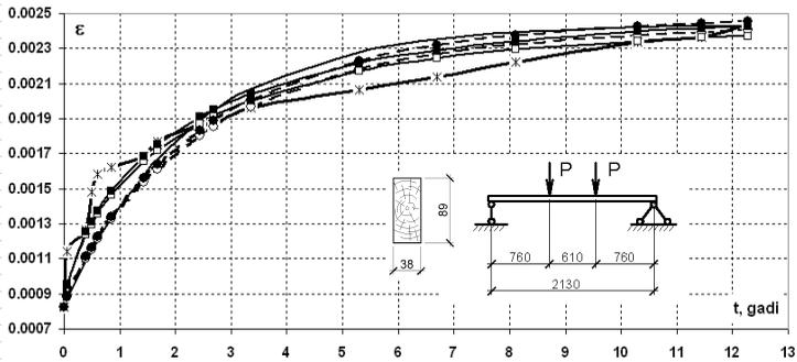
Fig 4.1. Loading scheme, cross-section and creep curves of Douglas-fir beam, if load  $P=0.526$  kN. Patterns applied in graphic:
