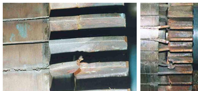
Fig. 2. Broken rotor bars due to heavy duty operation [5].
