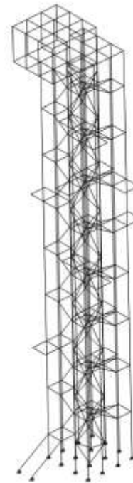
Fig.3. FE model of the tower
