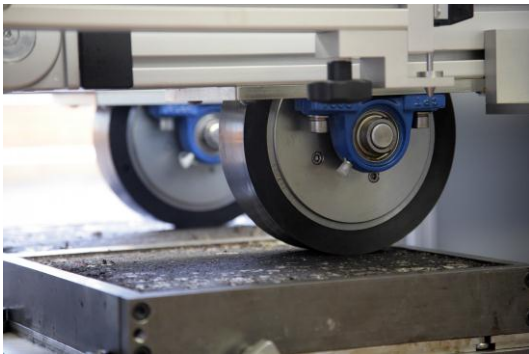
Fig 3. Test equipment for wheel tracking test
