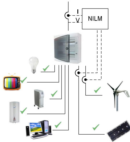
Fig. 3. Proposed solution with additional current sensors
