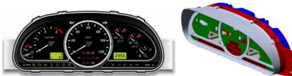
Figure 19. Design of the gage panel (GP) of enterprise Merpro , designed as AMO PLANT and 3D geometrical model
