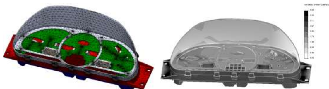
Figure 20. Meshed 3D model and von Mises stresses distribution in initial design of GP
