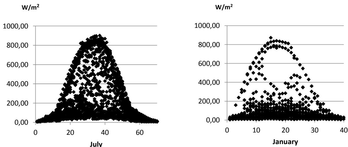
Fig. 2.3. The frequency of solar radiation in different times of the year
