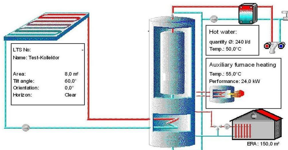
Fig.3.1. Simulation variant principal scheme of Solar combined system
