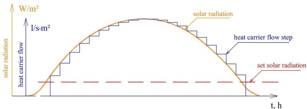
Fig. 4.1. Flow depending on the intensity of solar radiation
