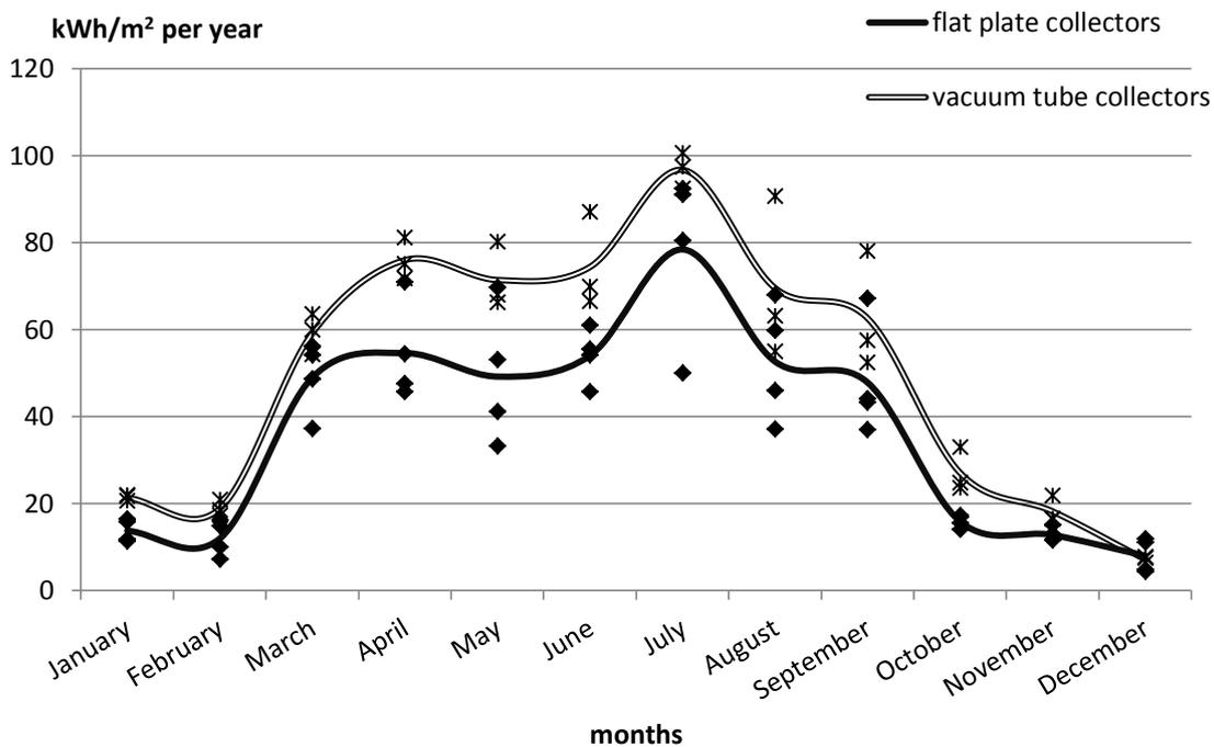
Fig. 2.5. Amount of energy produced by different types of collectors
