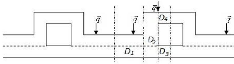
Fig. 2.7. Absorber plate cross section
