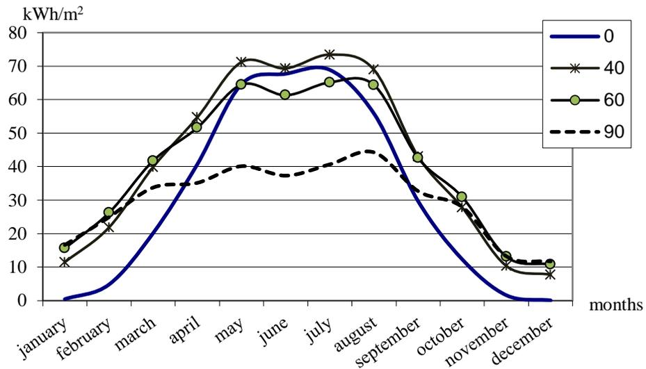
Fig. 2.6. The amount of solar energy, depending on the angular position of the collector
