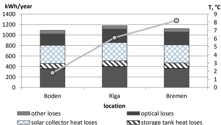
Fig.3.2. Heat losses volume depending on simulation variant location
