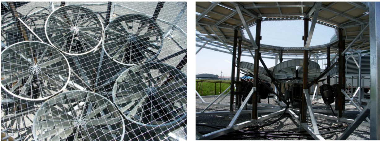
Fig. 10. Stationary installation with the system fans and not closed circuit and open work section.
