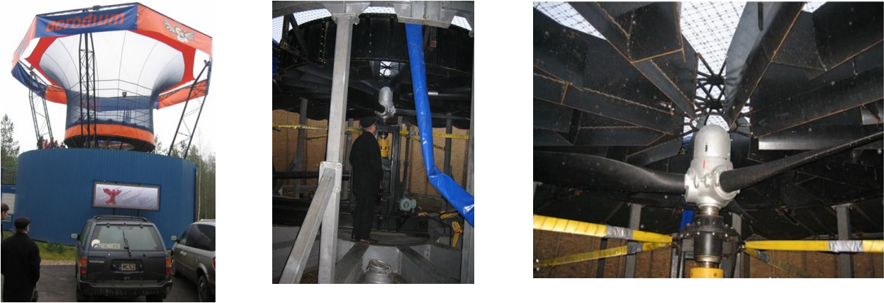
Fig. 8. Stationary aerodynamic stand with not closed circuit and open work section.
