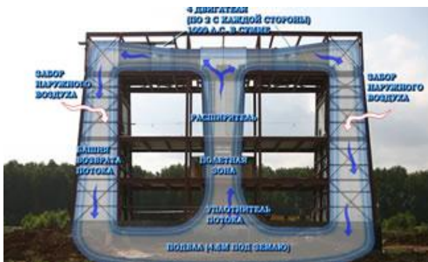
Fig.4. The closed type vertical wind tunnel for paratroopers training in the "Sky Venture"
