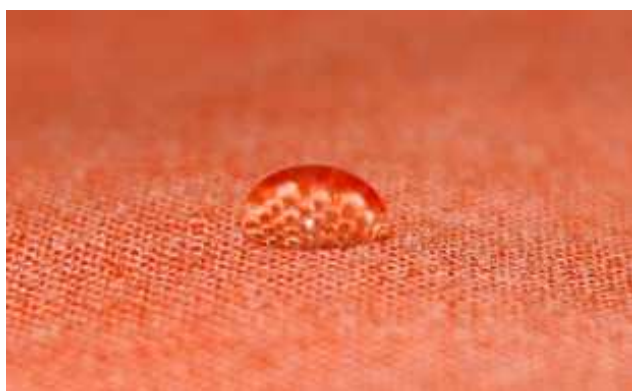
a Fig.3. Surface energy of different textiles – a: cotton 100% (C3); b: cotton 50% / polyester 50% (Co/PE 1)
