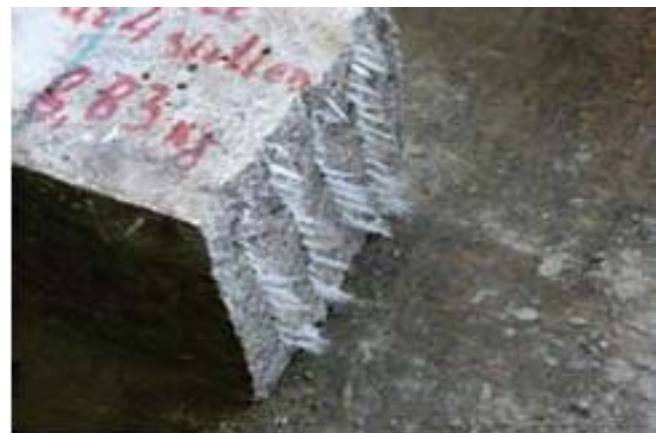
Fig.2. Concrete prisms reinforced by four glass fiber knitted fabrics. One half of the beam was broken under 4 –point bending.
