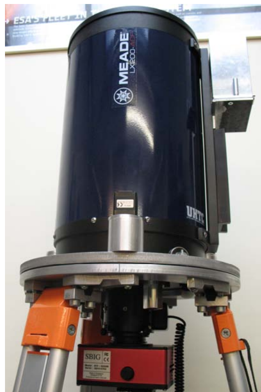
Figure 12. New digital zenith camera design
