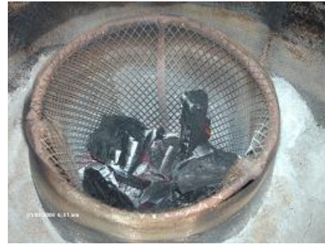
Fig.3. The incinerator converting rice husk into RHA
