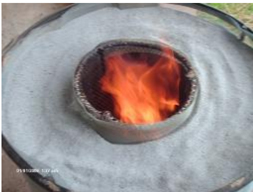
Fig. 2. Inner steel mesh basket charged with red hot charcoal
