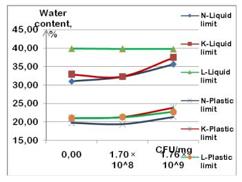
Fig 5. Comparative characterization of plastic and liquid limits of three illite clay samples K, L, N in dependence on bacteria Ps. Fluorescens AM PS11 concentrations.
