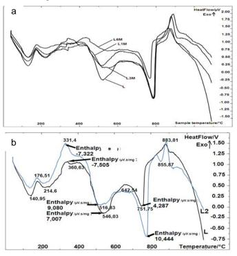
Fig. 3. DTA curves for: a - chemically untreated clay L and treated by 1M, 3M and 6M NaOH-water solution; b - microbiologically treated by bacteria Ps. fluorescens AM PS11: L - not treated, L2 - treated for 48h. \* - enthalpy unit of measurement for all points is μV.s/mg.
