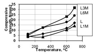
Fig. 6. Compressive strength in dependence on sintering temperature of ceramic samples achieved from differently treated L clay.
