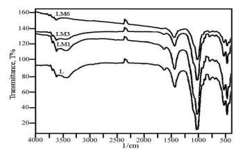
Fig.4. FTIR-spectra of clay L and treated by 1M, 4M and 6M NaOH solutions.
