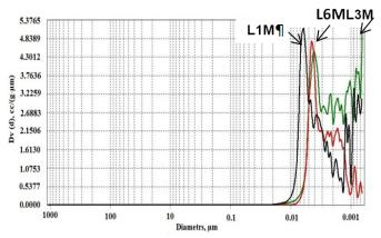
Fig. 7. Porosity development of sintered at 700°C ceramic sample L in dependence on molar concentration of NaOH solutions: L1M – raw clay L treated by 1M NaOH, L3M – by3M NaOH, L6M-by 6M NaOH.
