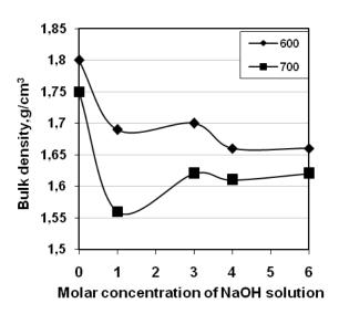
Fig.8. Bulk density of sintered ceramic sample L in dependence on molar concentration of NaOH solution.
