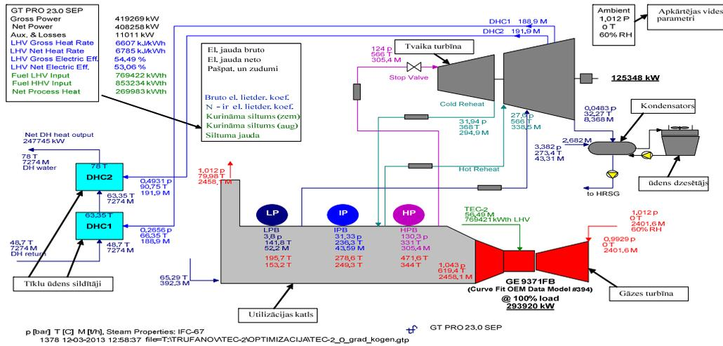
Fig.2.2. Structure of the model of CHPP-2 first power block (software Thermoflow environment)
