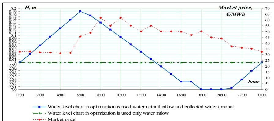
Fig.5.5. The changes in the water level realizing the optimization by means of the GRG method taking into account the market prices calculation
