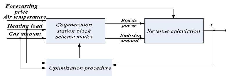
Fig.2.1 Combined heat power plant model's generalized flow-chart
