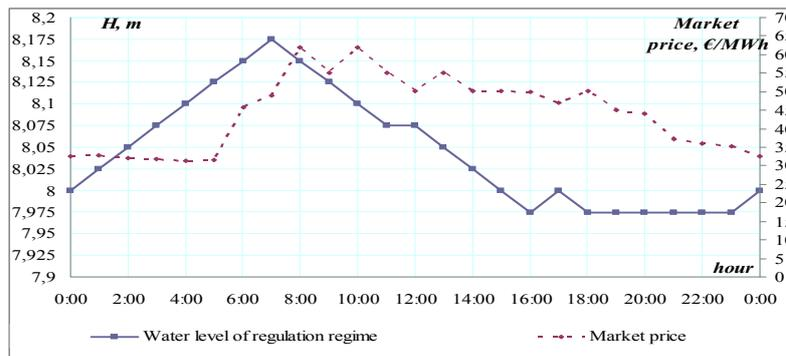
Fig.5.1. The level of water realizing optimization by means of DP method and step 0,025m
