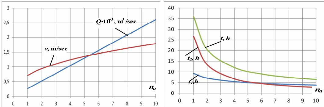
Fig.2.4. Dependence of the values on the amount of Pļaviņas HPP started up aggregates
