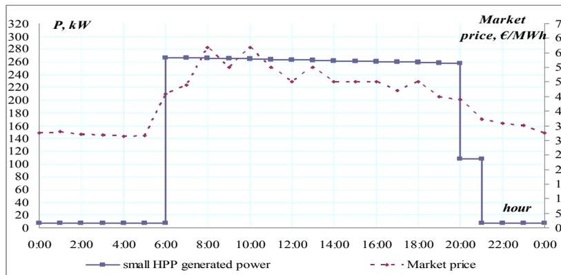
Fig. 5.4. The generating power realizing optimization by means of DP method and step 0,01m
