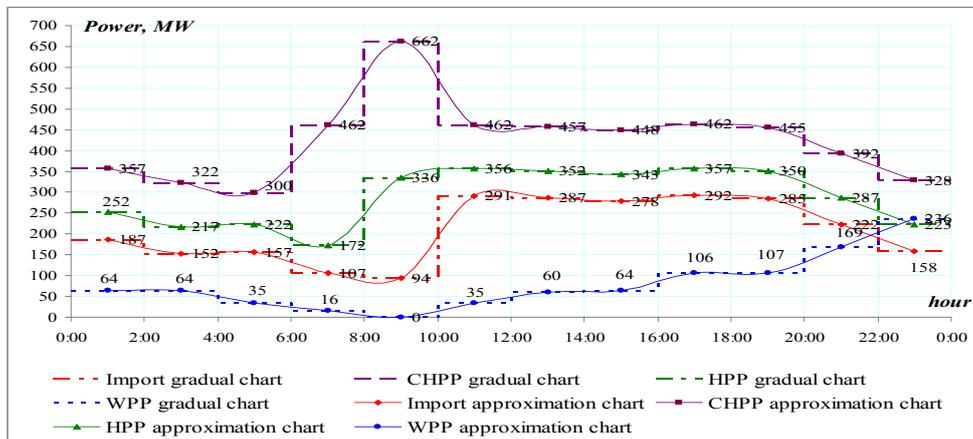
Fig.4.9. The distribution of the power among stations taking into account the station input/output electrical market component
