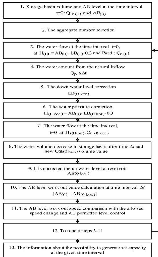
Fig. 2.5. Flow-chart of the hydro electric station model
