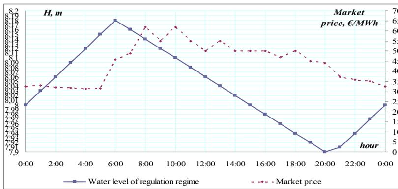
Fig. 5.2. The level of water realizing optimization by means of DPmethod and step 0,01m
