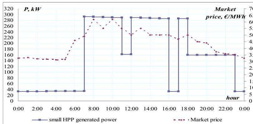
Fig.5.3. The generating power realizing optimization by means of DP method and step 0,025m
