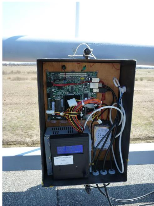
Fig. 5.18. One of the first versions of the gateway (installed at a nursing home "Selga" roof)
