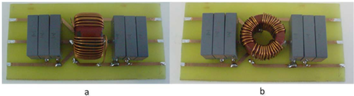
Fig. 3.4. a) Filter prototype with vertical CM choke b) Filter prototype with horizontal CM choke
