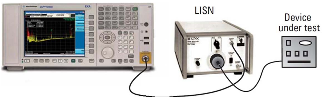
Fig. 1.5. Conducted emission measurements according to EN 55011
