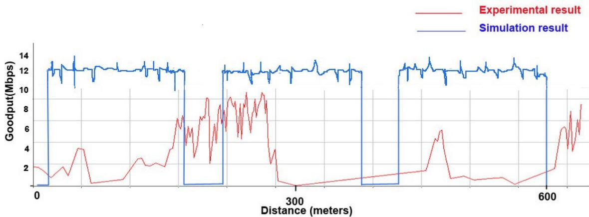
Figure 5.5. Goodput comparison with experimental and simulation results at 90 km/h
