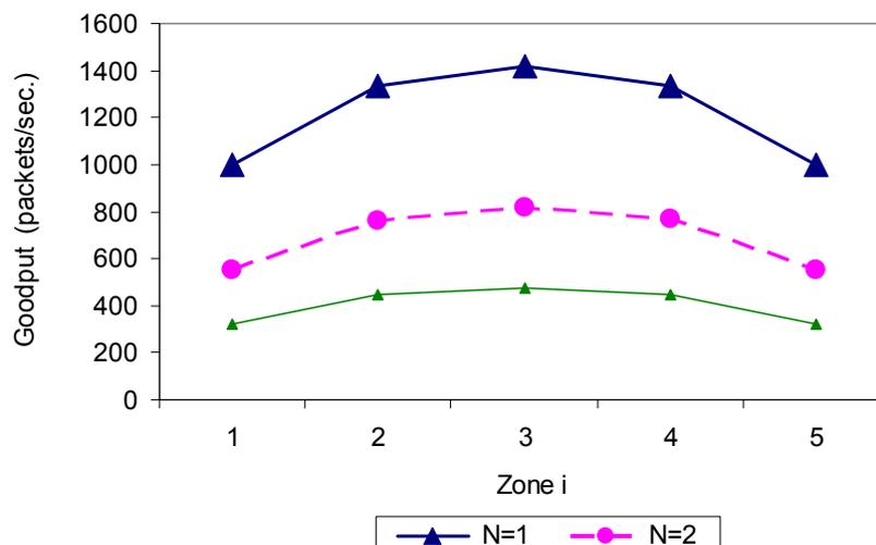
Figure 3.5. Goodput in wireless network with one router depending on distance for 802.11n
