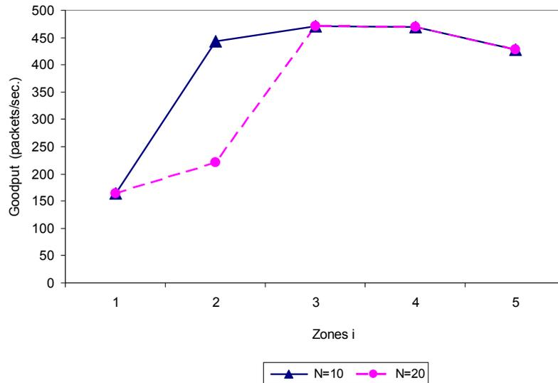
Figure 3.7. Goodput for a two-stage network model with  $P_{10} = 0.999$   $P_{12} = 0.001$  for 802.11n and LTE
