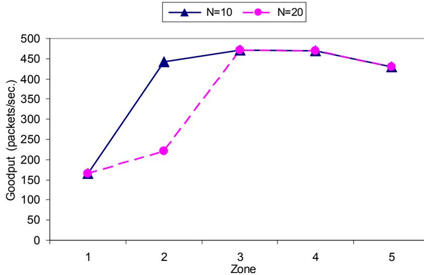
Figure 3.4. Goodput for moving with 10 and 20 vehicles
