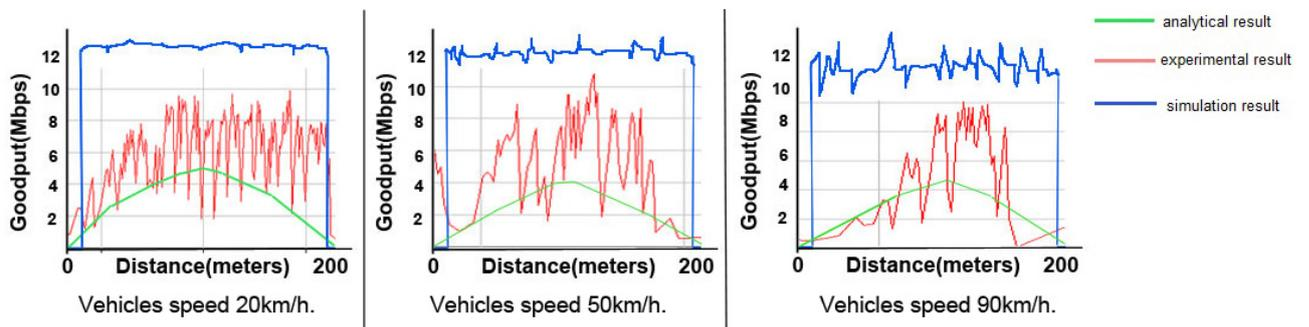
Figure 5.6. Goodput comparison with experimental, simulation and analytical results for vehicles speed 20-90 km/h
