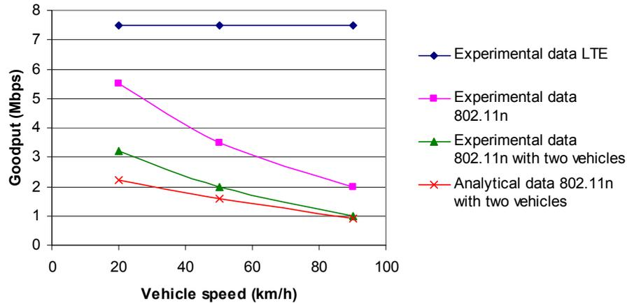
Figure 5.7. Goodput productivity dependence on the vehicle speed
