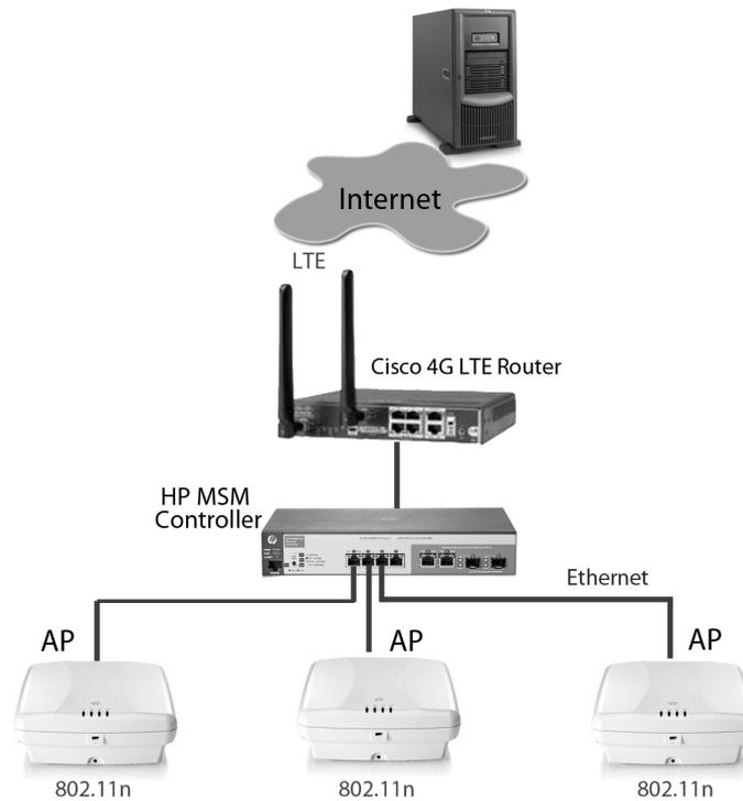
Figure 4.1. Two-stage network model
