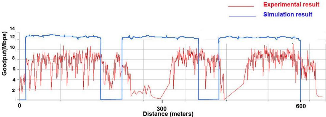
Figure 5.3. Goodput comparison with experimental and simulation results at 20 km/h
