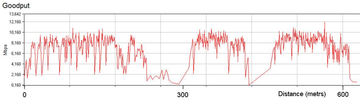
Figure 4.2. Two-stage goodput with 4G and 802.11n at speeds of 20 km/h
