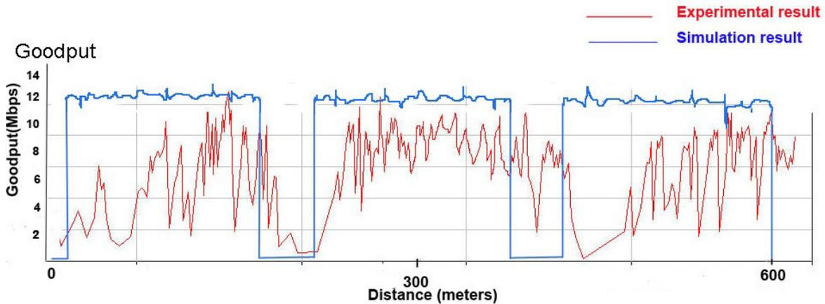
Figure 5.4. Goodput comparison with experimental and simulation results at 50 km/h
