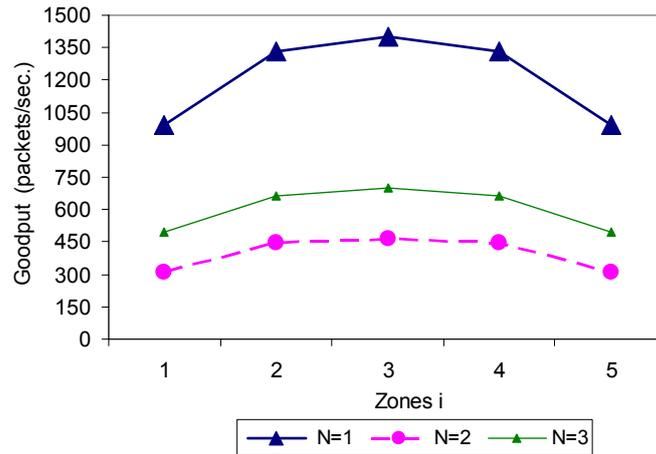
Figure 3.8. Goodput for a two-stage network model with  $P_{10} = 0.999$   $P_{12} = 0.001$  for 802.11n and LTE at the Erlang distribution
