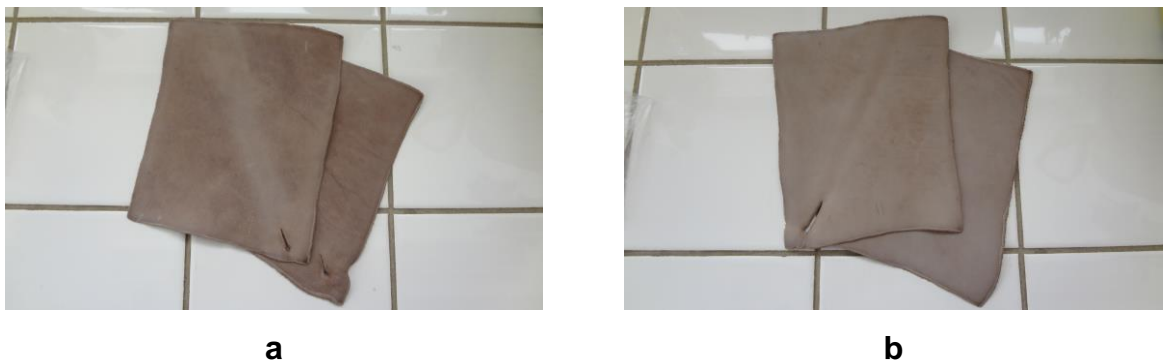
Figure 4.17 Leather produced from hide stored in vacuum (a – 5 days; b – 19 days)
