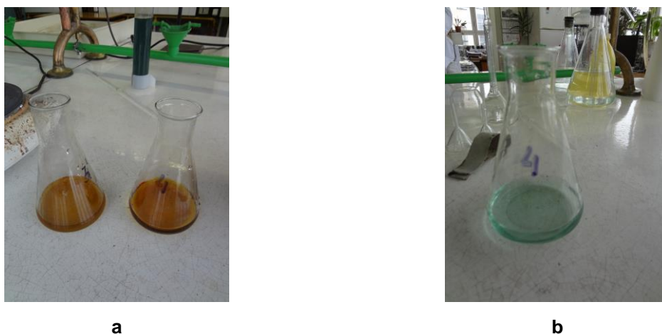
Figure 3.14 Process of determination of chromium oxide concentration in solution: a -test solution before titration [APF]; b -test solution after titration [APF]
