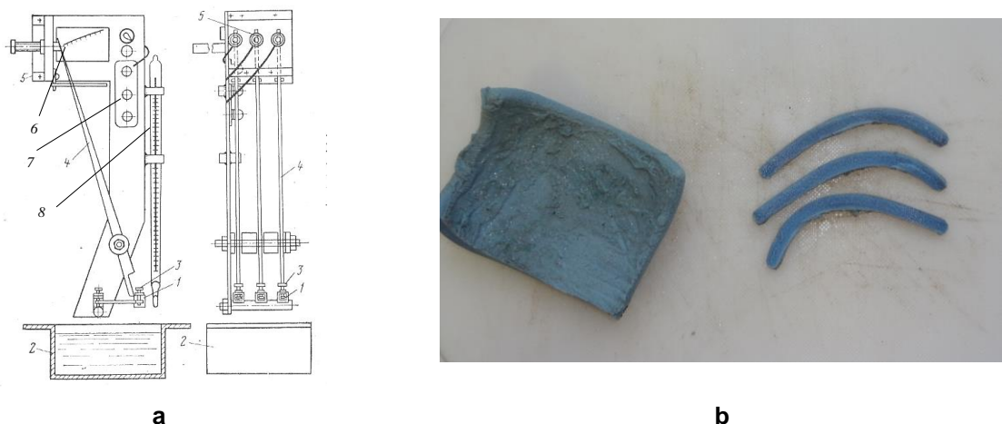
Figure 3.11 Equipment for determination of shrinkage temperature over 100^{\circ}\text{C} : a -scheme of shrinkage temperature apparatus (1-jaws; 2-pot with glycerol; 3-lower regulative screw; 4-heaver; 5-upper regulative screw; 6-contacts; 7-indicating lamps; 8-thermometer.) [67] b -wet blue test piece and strips for shrinkage temperature determination [APF]
