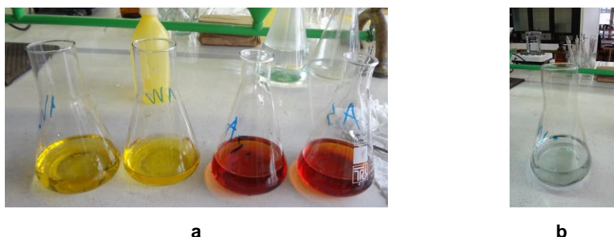
Figure 3.15 Process of determination of chromic oxide content in leather: a -left flasks after last boiling, right flasks after adding potassium iodide solution [APF]; b -flasks after titration process [APF]
