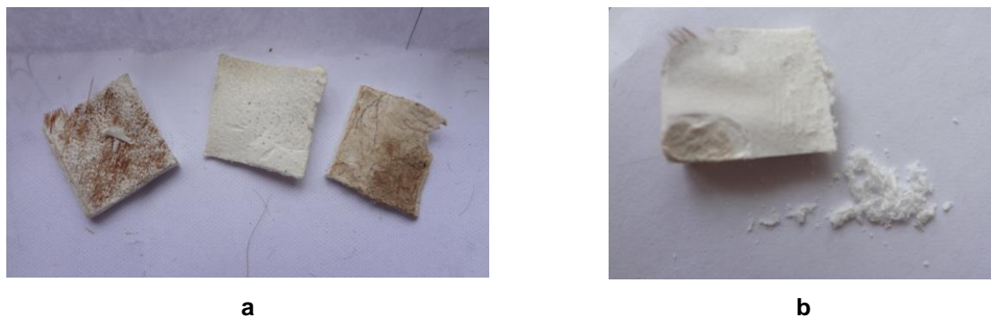
Figure 3.18 a-sample cut in three pieces for IR analysis [APF]; b-hide powder for DSC analysis [APF]
