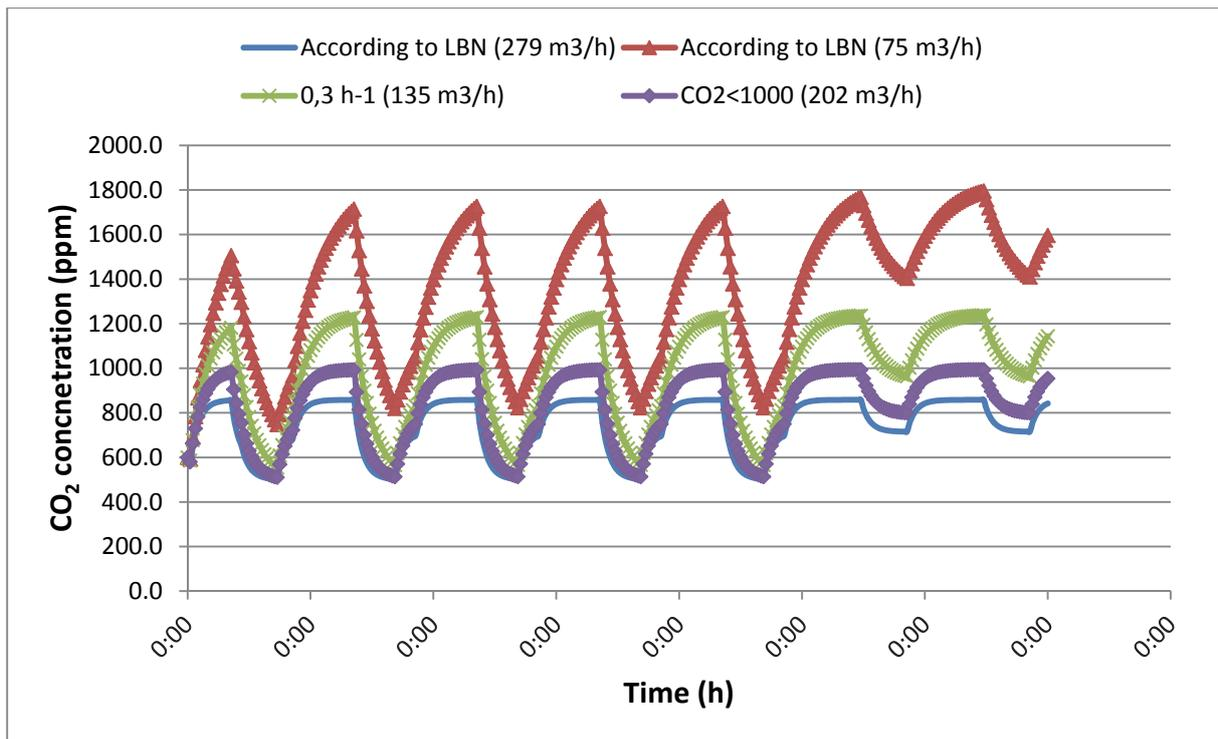
Fig. 4-2: CO<sub>2</sub> level (ppm) in the building during a week at different volumes of ventilation air.
