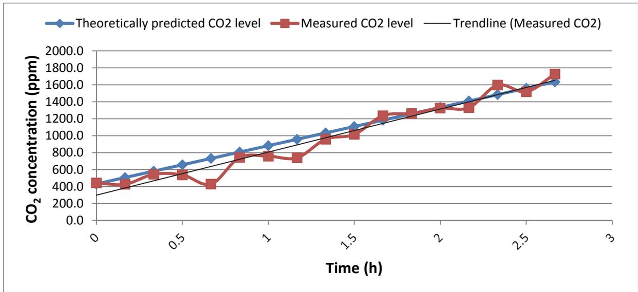
Fig. 3-2: The predicted and measured CO<sub>2</sub> concentration inside the climatic chamber with adjusted CO<sub>2</sub> production rate.
