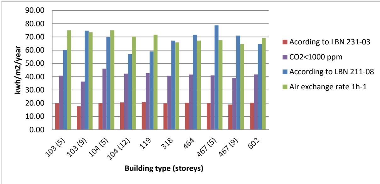
Fig. 4-1: Comparison of calculated energy consumption necessary for air heating of ventilation air to the total area (kWh/m<sup>2</sup>/year).
