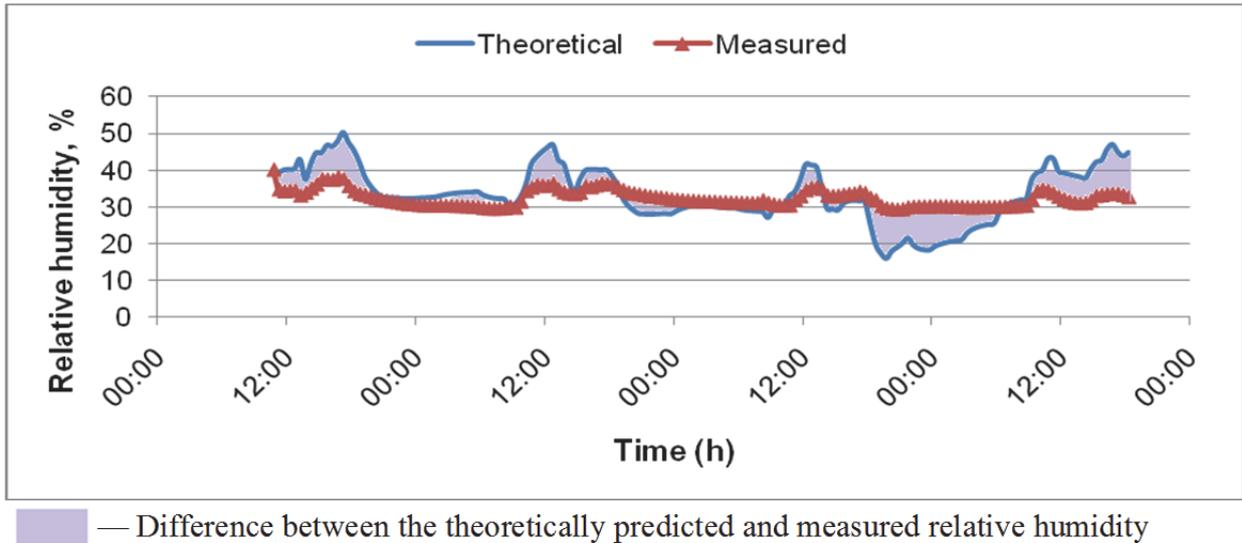
Fig. 3-5: The theoretically predicted and measured relative humidity in the office with 3 persons and 30 m<sup>2</sup> area during time period of 29/03/2011 to 01/04/2011.
