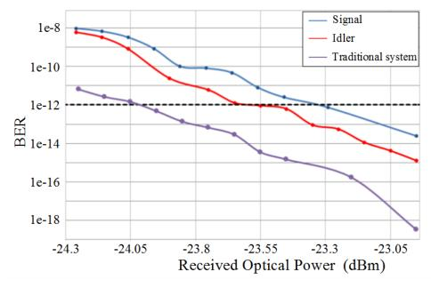
*Fig.23*. BER value dependence on the power of the detected signal in the standard singlechannel system (violet) and in the 1<sup>st</sup> channel of the system with the chosen FOPA configuration of the signal at its initial frequency (blue) and of the idler (red).
