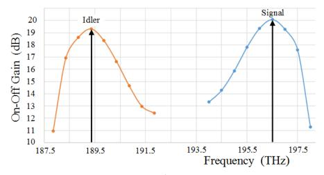
*Fig. 22.* FOPA produced on-off gain for the 1<sup>st</sup> channel at idler frequencies (orange line) and at the initial signal frequencies (blue line).
