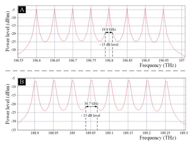
*Fig. 10.* Spectra of the amplified signal (A) and the generated idlers (B) at the output of the single-pump FOPA.
