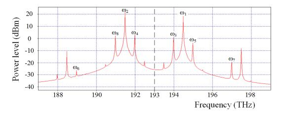
*Fig. 11.* Optical spectrum at the output of a dual pump FOPA with 200 mW 191.5 THz pumps and 500 meter long HNLF.
