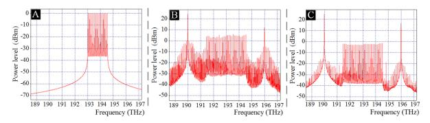
*Fig.13.* Optical spectrum at the input of the FOPA when initial carrier power is set to 0 dBm (a), and optical spectra at the output of the HNLF when the power of the initial carriers is set to 0 dBm (b) and to -10 dBm (c).
