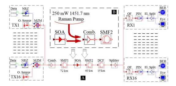
*Fig.* 7. Simulation model of the 16-channel 10 Gbps DWDM transmission system with the SOA inline amplifier (a) or with a hybrid Raman-SOA amplifier (b).
