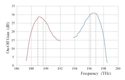
*Fig. 19.* Gain spectrum ensured by the FOPA with 790 mW 1554.15 nm linearly polarised pumping radiation at initial signal frequencies (blue line) and idler frequencies (red line).
