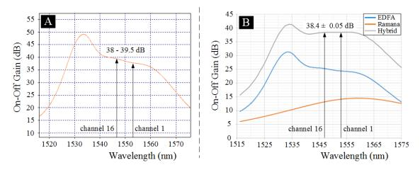
*Fig. 5.* Gain spectra of the EDFA inline amplifier (A) and of the hybrid Raman-EDFA amplifier (B).
