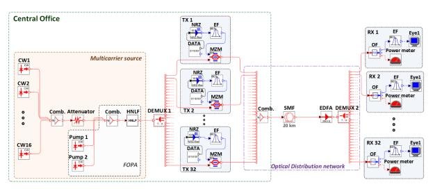
*Fig. 12.* Simulation model of the 32 channel 10 Gbps WDM transmission system with the provided multicarrier source solution, which is based on wavelength conversion using a dual-pump FOPA.
