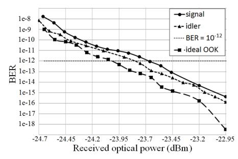
*Fig. 17.* BER value dependence on the detected signal power in the standard single-channel transmission system (dashed line), and in the system with modulation format conversion at the initial signal frequency (solid line) and at idler frequency (dotted line).
