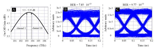
*Fig. 8.* DRA produced gain spectrum (a) and eye diagrams of the  $9^{th}$  channel in the system with the SOA inline amplifier (b) and the  $10^{th}$  channel in the system with the Raman-SOA hybrid amplifier (c).
