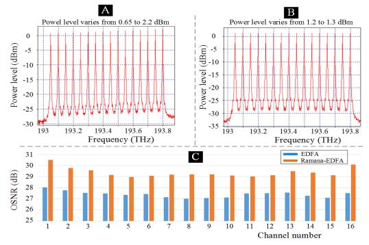
*Fig. 6.* Signal spectra at the output of the EDFA (a) and at the output of the hybrid Raman-EDFA amplifier (b), and OSNR comparison among all 16 channels in the system with the EDFA inline amplifier and the hybrid Raman-EDFA amplifier (c).
