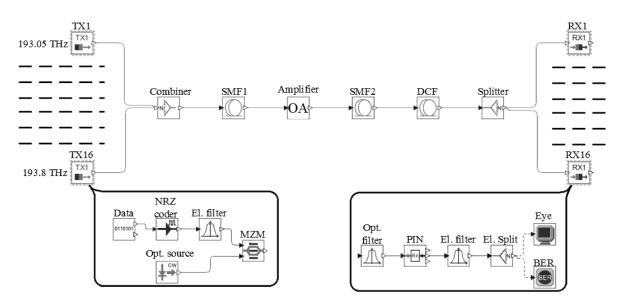
*Fig.2.* Simulation model of the 16-channel 10 Gbps DWDM transmission system used for comparison of optical amplifier performance.
