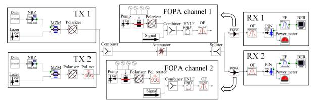
*Fig. 21.* Simulation model of the two-channel optical transmission system with FOPA for division and amplification of polarisation multiplexed signals.
