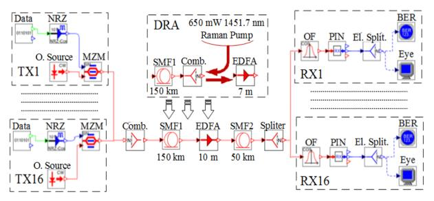
*Fig. 4.* Simulation model of the 16-channel 10 Gbps DWDM transmission system with an EDFA inline amplifier or with a hybrid Raman-EDFA amplifier.
