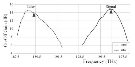
*Fig. 16.* Gain spectrum produced by the single-pump FOPA with linearly polarised pumping radiation at signal frequencies (solid line) and at idler frequencies (dotted line).
