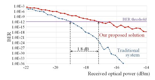
*Fig. 14.* BER value dependence on the power of the detected signal for the 12<sup>th</sup> channel in the system with the proposed multicarrier source solution (red line) and in the system with traditional architecture (blue line).
