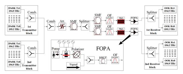
*Fig. 18.* Simulation model of the 16-channel WDM transmission system with two access network branches, where in each branch the FOPA pre-amplifier is used for 2PolSK to NRZ-OOK modulation format conversion.
