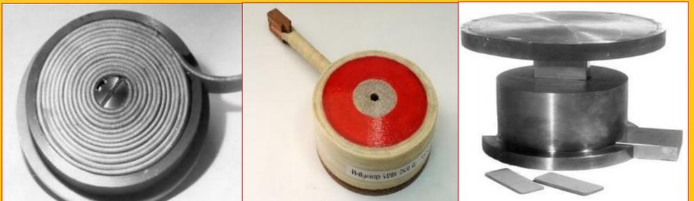
Flat-coil, cylindrical coil and form for the CCPM.
